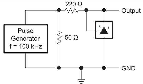
Figure 12. Test Circuit for Pulse Response
