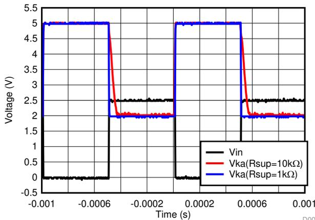
Figure 24. Output Response With Various Cathode Currents
