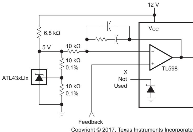
Figure 36. PWM Converter With Reference
