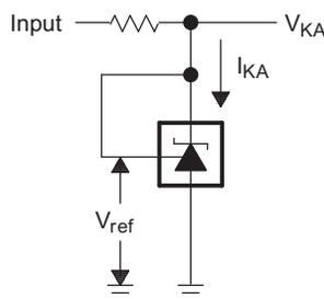
Figure 17. Test Circuit for  $V_{KA} = V_{ref}$
