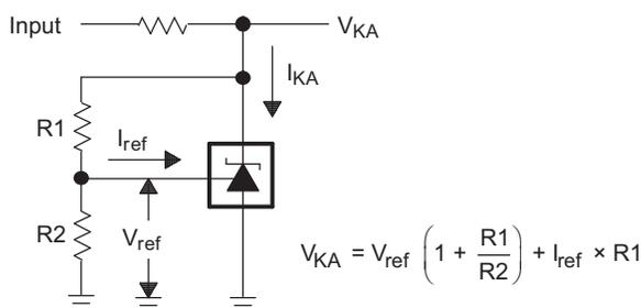
Figure 18. Test Circuit for  $V_{KA} > V_{ref}$
