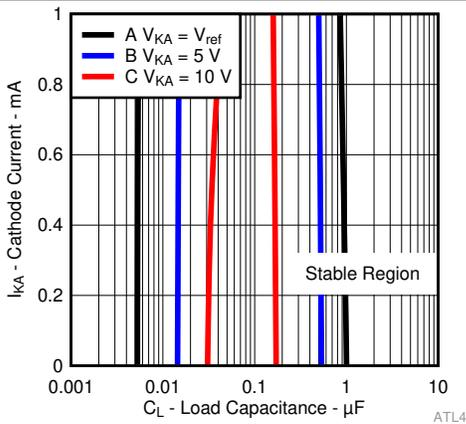
The areas in-between the curves represent conditions that may cause the device to oscillate. For curves B, and C,  $R_2$  and  $V_+$  are adjusted to establish the initial  $V_{KA}$  and  $I_{KA}$  conditions, with  $C_L = 0$ .  $V_{BATT}$  and  $C_L$  then are adjusted to determine the ranges of stability.
