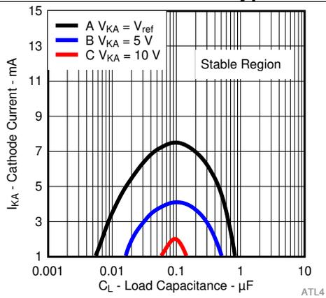
The areas under the curves represent conditions that may cause the device to oscillate. For curves B and C,  $R_2$  and  $V_+$  are adjusted to establish the initial  $V_{KA}$  and  $I_{KA}$  conditions, with  $C_L = 0$ .  $V_{BATT}$  and  $C_L$  then are adjusted to determine the ranges of stability.
