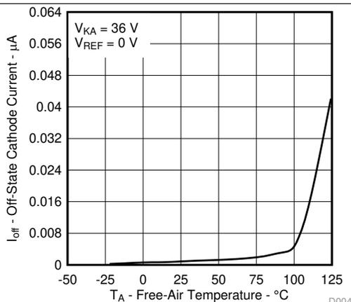
Figure 5. Off-State Cathode Current vs Free-Air Temperature
