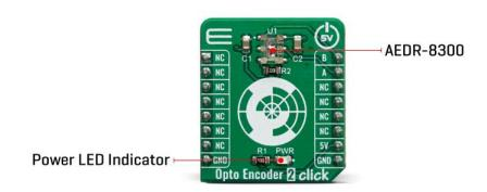
Opto Encoder 2 click offers options of either single channel or two-channel quadrature digital outputs. Being TTL compatible, the outputs of the AEDR-8300 series can be interfaced directly with MCU. Hence the Opto Encoder 2 click provides great design-in flexibility and easy integration into existing systems. A and B pins are routed to the routed to the mikroBUS™ PWM and INT pins, thus providing the quadrature digital signal.
