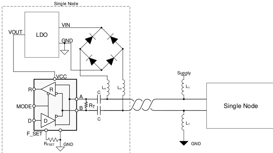
Figure 9-1. Typical power line network with 2 nodes
