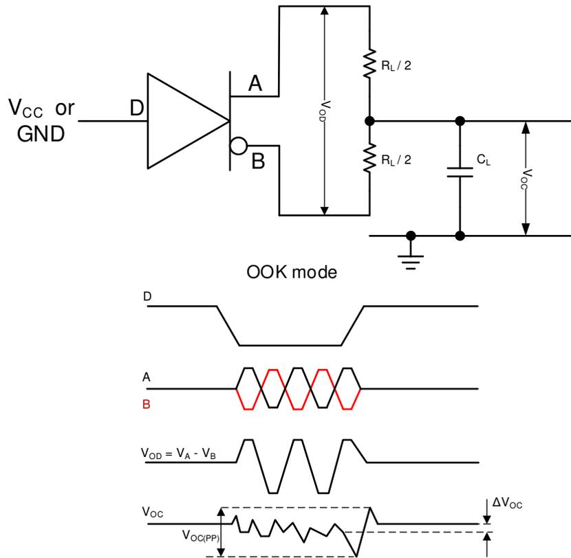
**Figure 7-2. Measurement of Driver Differential and Common-Mode Outputs**
