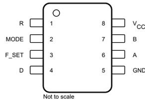
**Figure 5-1. DRL Package, 8-Pin SOT-23, Top View**
