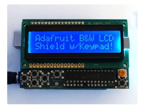
This shield is perfect for when you want to build a stand-alone project with its own user interface. The 4 directional buttons plus select button allows basic control without having to attach a bulky computer.
