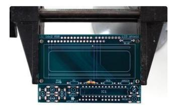
We'll start with the first resistor R1 - which has yellow, violet, red, gold bands on it. This resistor is part of the interface between the Arduino and the 'port expander' that controls the LCD.
