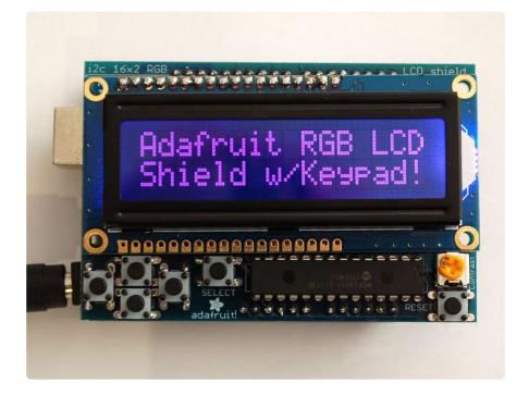
With this in mind, we wanted to make it easier for people to get these LCD into their projects so we devised a shield that lets you control a 16x2 Character LCD, up to 3 backlight pins AND 5 keypad pins using only the two I2C pins on the Arduino! The best part is you don't really lose those two pins either, since you can stick i2c-based sensors, RTCs, etc and have them share the I2C bus. This is a super slick way to add a display without all the wiring hassle.
