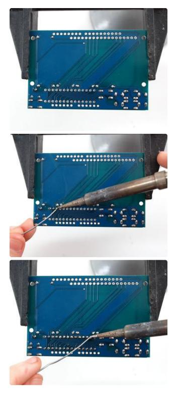
Flip over the PCB and solder in the three legs of the potentiometer and then all 28 pins of the port expander.
