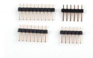
Take a stick of 36 pin header and break off a 10 pin piece, an 8 pin piece and two 6 pin pieces.
