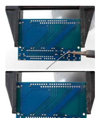
Solder each leg, taking care not to accidentally 'short' two button legs together. The ones for the directional pads are very close!
