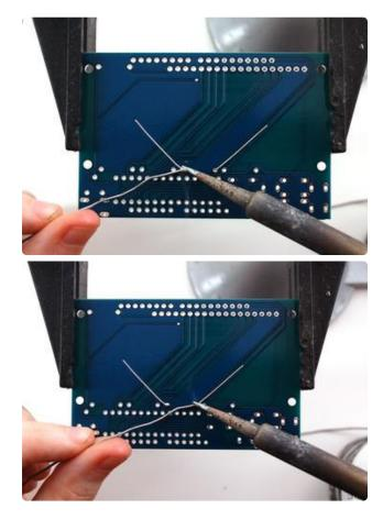
With your soldering iron heated up and ready, solder in both leads of the resistor. To do this, heat up the round ring pad and the wire lead at the same time for 2 or 3 seconds, then dip the end of the solder into the heated joint to melt it in.
