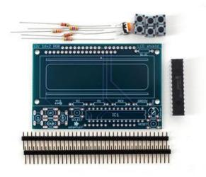
Check the kit against the parts list () to verify you have all the parts necessary
