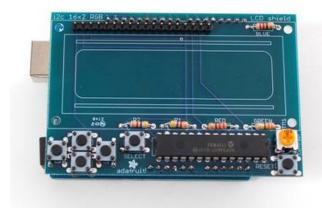
Next, check if you have an RGB LCD (with 18 pins) or a Monochrome display (not RGB, with 16 pins).
