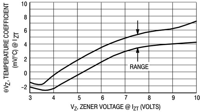
Figure 2. Temperature Coefficient-Range for Units 3 to 10 Volts
