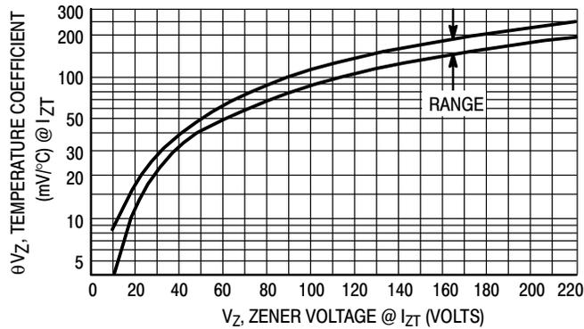
Figure 3. Temperature Coefficient-Range for Units 10 to 220 Volts
