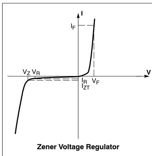
**ELECTRICAL CHARACTERISTICS** ( $T_A = 25^\circ\text{C}$  unless otherwise noted,  $V_F = 1.2\text{ V Max @ } I_F = 1.0\text{ A}$  for all types)
