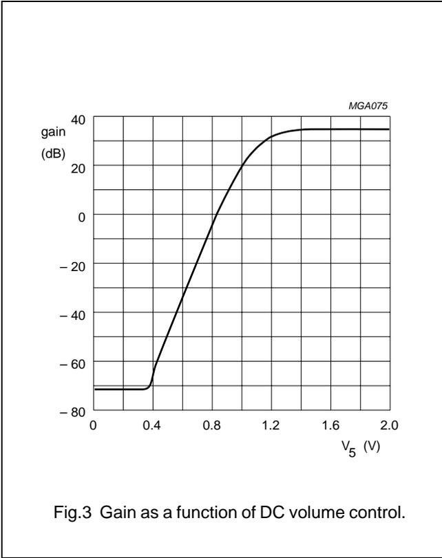
Fig.3 Gain as a function of DC volume control.
