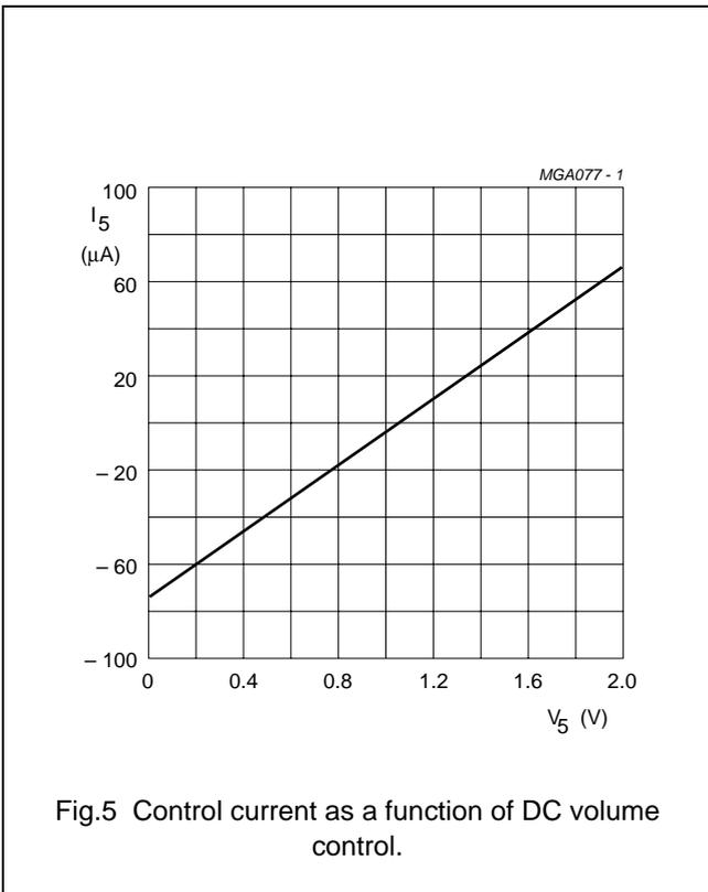
Fig.5 Control current as a function of DC volume control.
