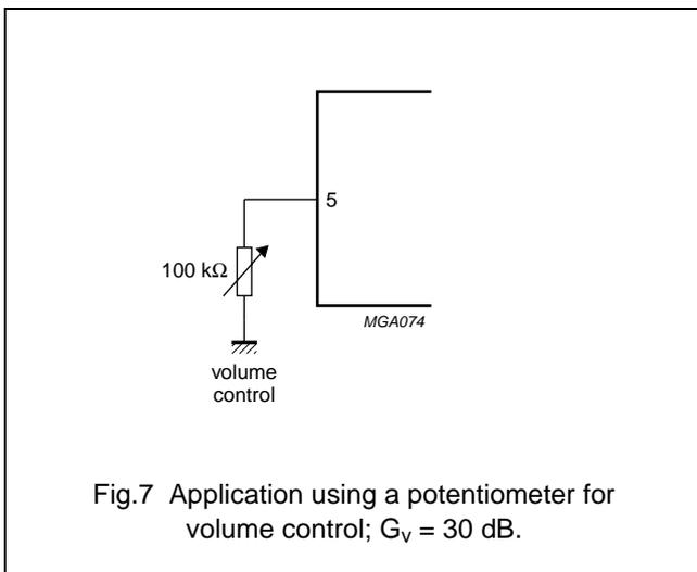
3 W BTL mono audio output amplifier with DC volume control
