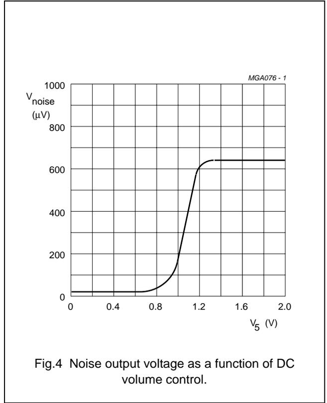
Fig.4 Noise output voltage as a function of DC volume control.
