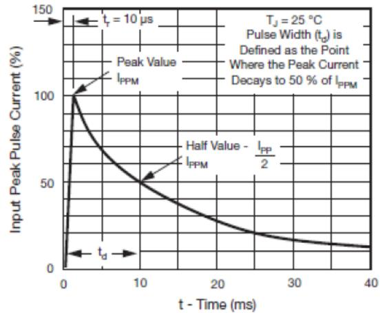
Fig. 3 - Pulse Waveform
