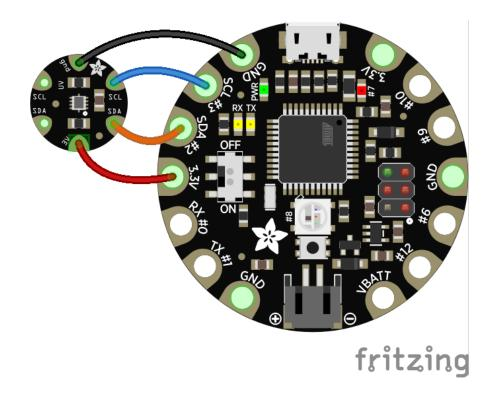
The SI1145 has a fixed I2C address (0x60), you can only connect one sensor per microcontroller!
