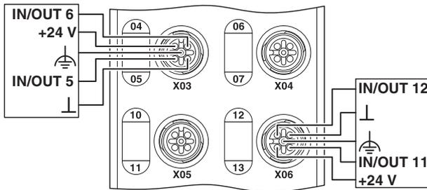
Figure 7 Example of connection of sensors and actuators
