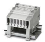
COMBI receptacle, Connection method: Push-in connection, Number of positions: 12, Cross section: 0.14 mm<sup>2</sup> - 1.5 mm<sup>2</sup>, AWG: 26 - 14, Width: 42 mm, Height: 27.1 mm, Color: gray, Mounting type: NS 35/15, NS 35/7,5
