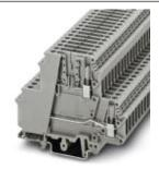
Disconnect terminal block, Connection type: Screw connection, Cross section: 0.2 mm² - 4 mm², AWG: 24 - 12, Nominal current: 26 A, Nominal voltage: 400 V, Length: 80 mm, Width: 6.2 mm, Color: blue, Assembly: NS 35/7,5, NS 35/15, NS 32
