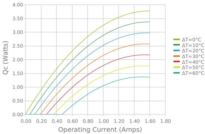
Heat Pumped at Cold Side
