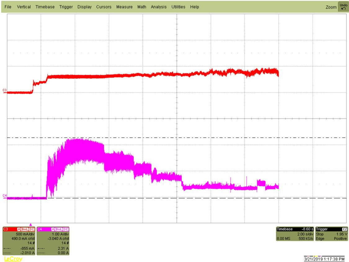
Figure 4. 2TB Typical startup and operation current profile
