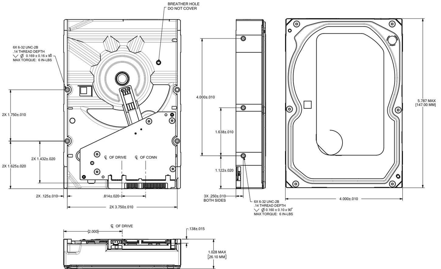
**Figure 7. Mounting configuration dimensions 4TB and 2TB models**
