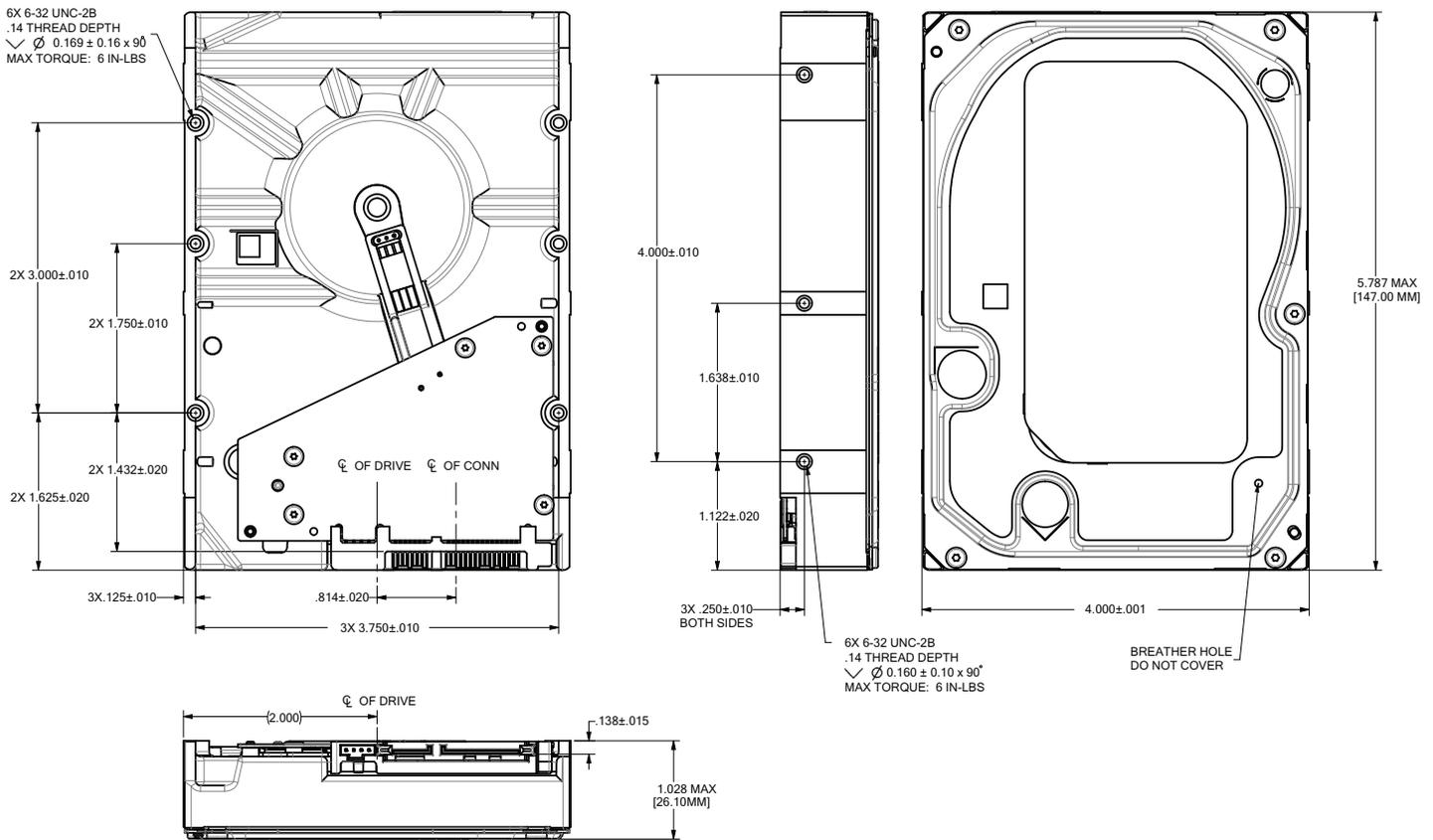
**Figure 6. Mounting configuration dimensions 8TB and 6TB models**
