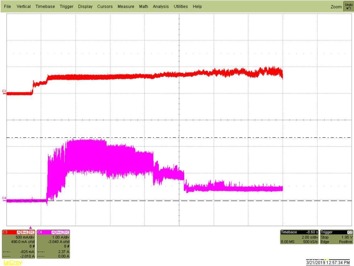
Figure 1. 8TB Typical startup and operation current profile
