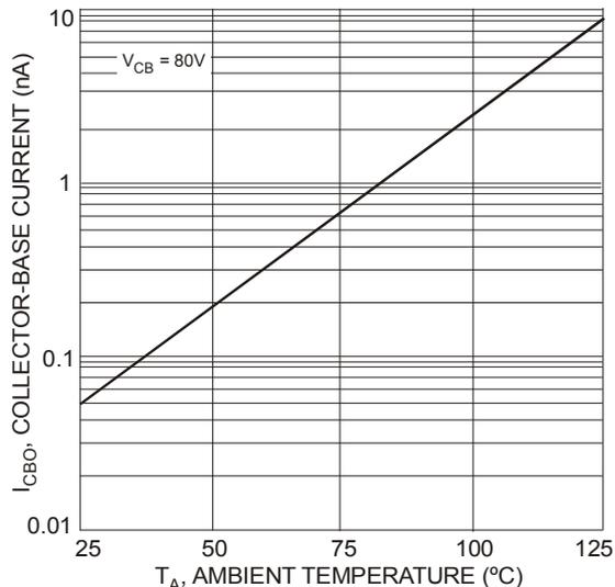
Figure 5 Typical Collector-Cutoff Current vs. Ambient Temperature
