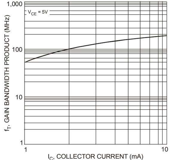
Figure 4 Typical Gain Bandwidth Product vs. Collector Current
