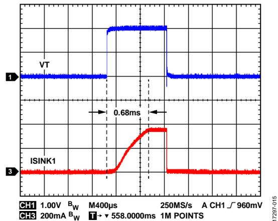
Figure 15. VT Speed During LED Current Pulsing
