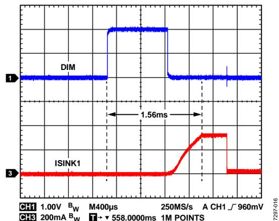
Figure 16. ISINK1 Response in 1 ms Pulse with DIM
