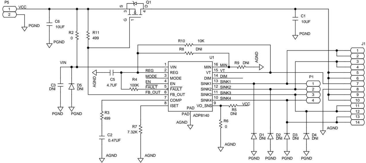
Figure 17. ADP8140EB-EVALZ Schematic
