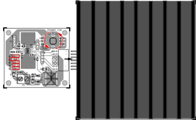
Figure 5. LED Current Reduction
