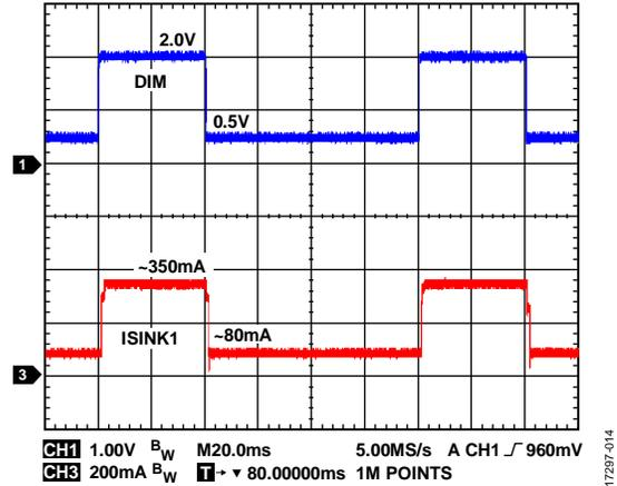
Figure 14. DIM Flexibility During LED Current Pulsing
