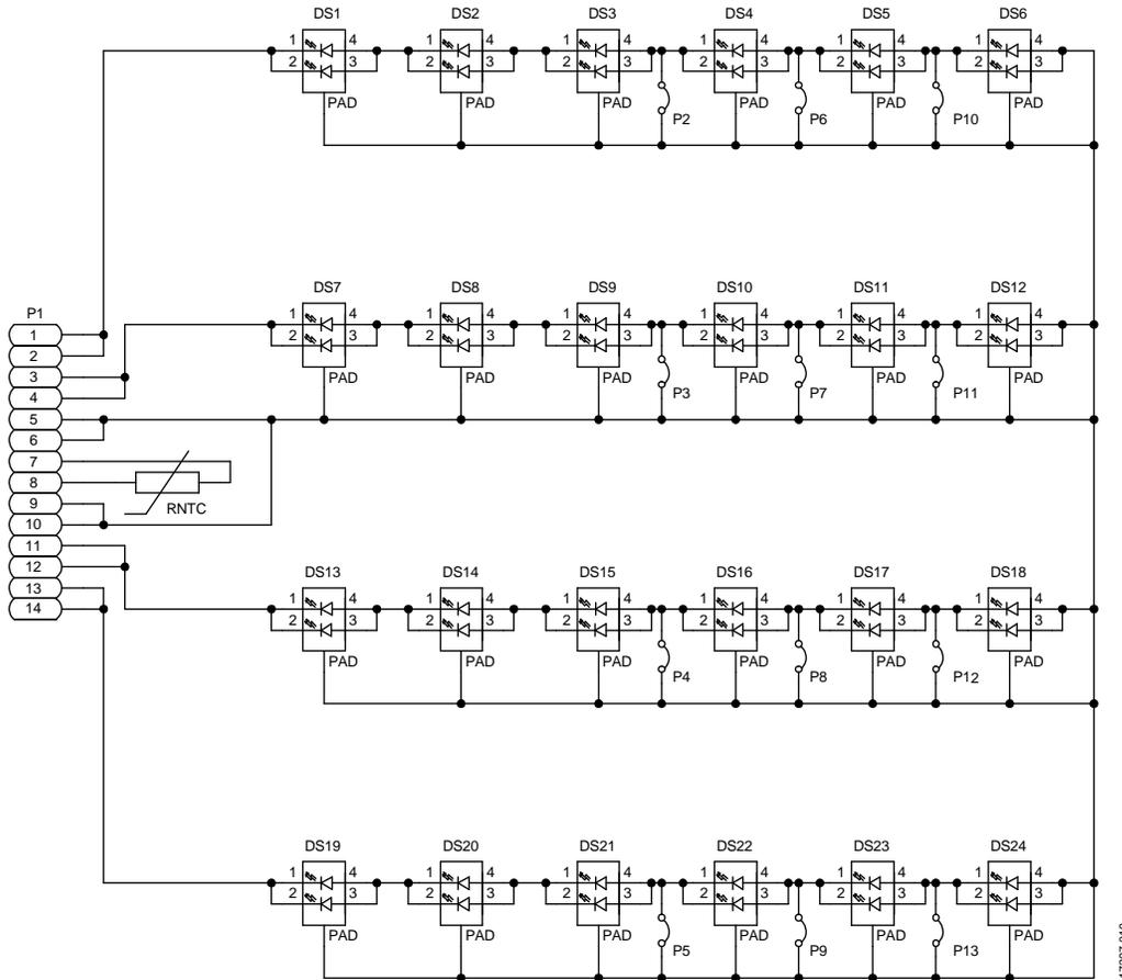
Figure 19. ADP8140 LED-EVALZ Schematic Connectors and Peripherals
