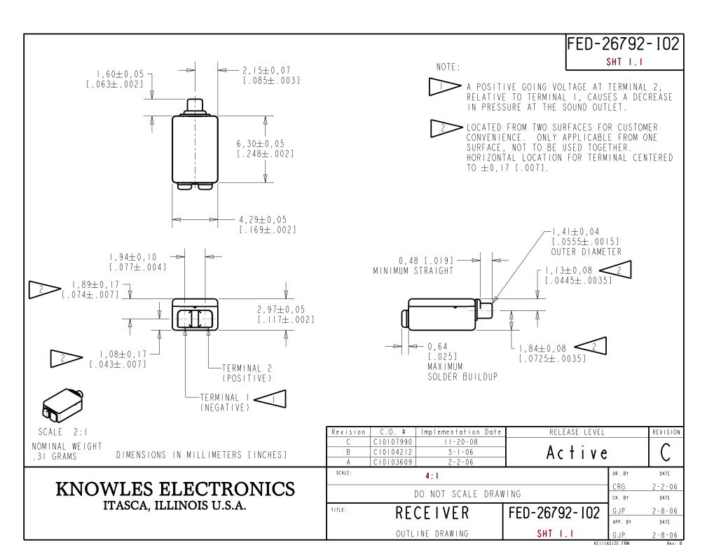
THE FED-26792-102 IS A FERROFLUID DAMPED ED-27305 RECEIVER WITH A PEAK OF 2dB RELATIVE TO THE SENSITIVITY AT IKHZ UNDER CONSTANT VOLTAGE DRIVE CONDITIONS.
