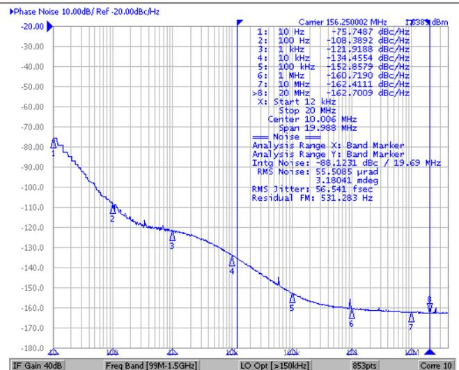
Jitter = 56 fs RMS (12 kHz to 20 MHz)
