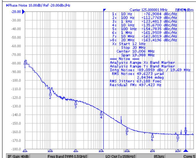
Jitter = 63 fs RMS (12 kHz to 20 MHz)
