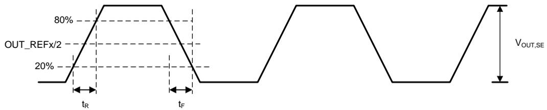
Figure 5. Single-Ended Output Voltage and Rise/Fall Time
