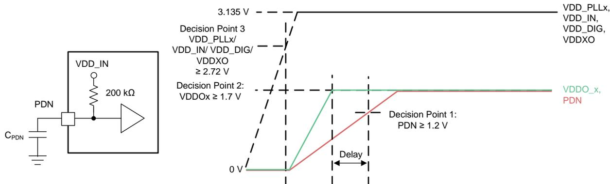
Figure 63. Recommendation for Power Up From Split-Supply Rails
