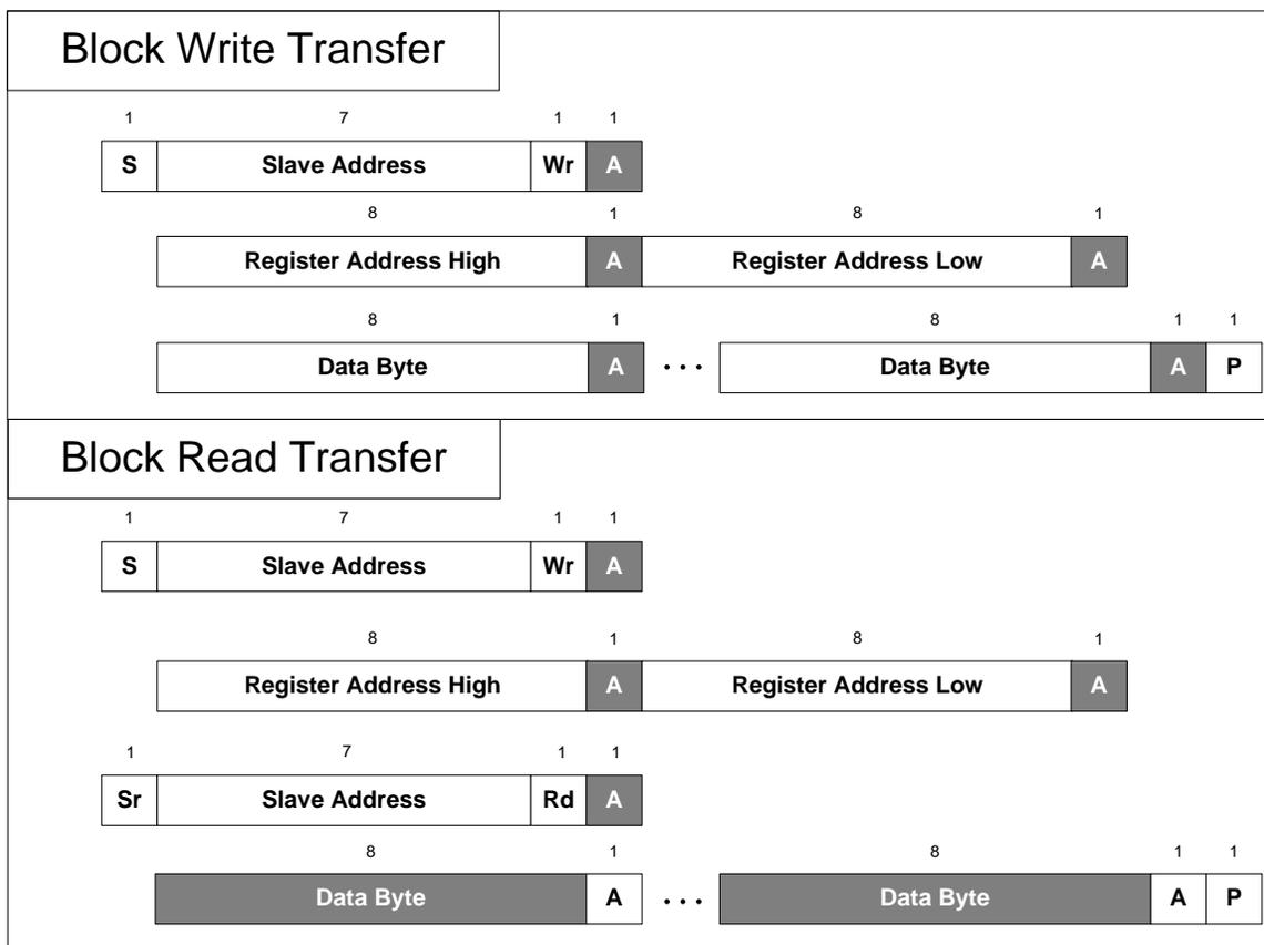
Figure 59. I<sup>2</sup>C Block Register Transfers
