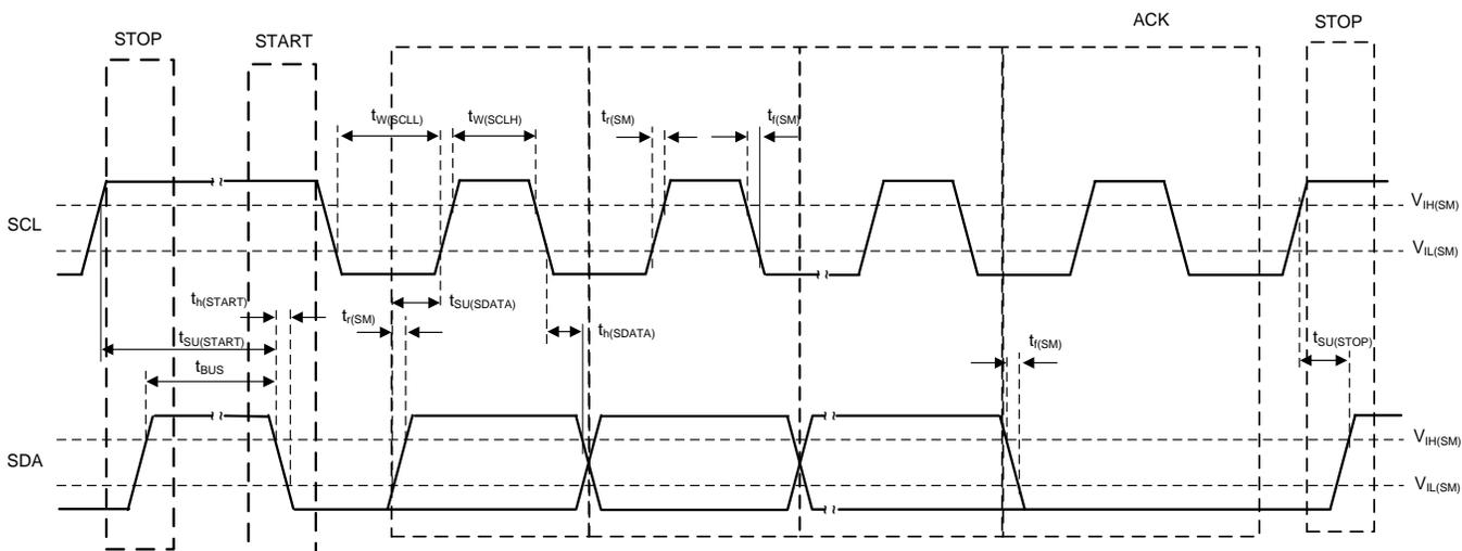
Figure 3. I<sup>2</sup>C Timing Diagram
