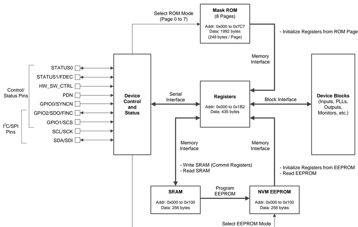
Figure 57. Device Control, Register, and Memory Interfaces
