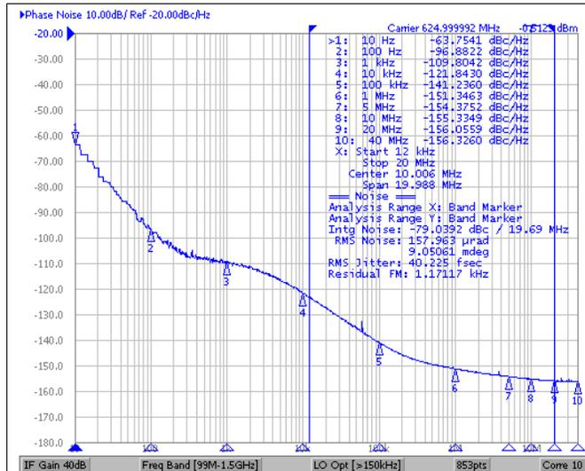
Jitter = 40 fs RMS (12 kHz to 20 MHz)
