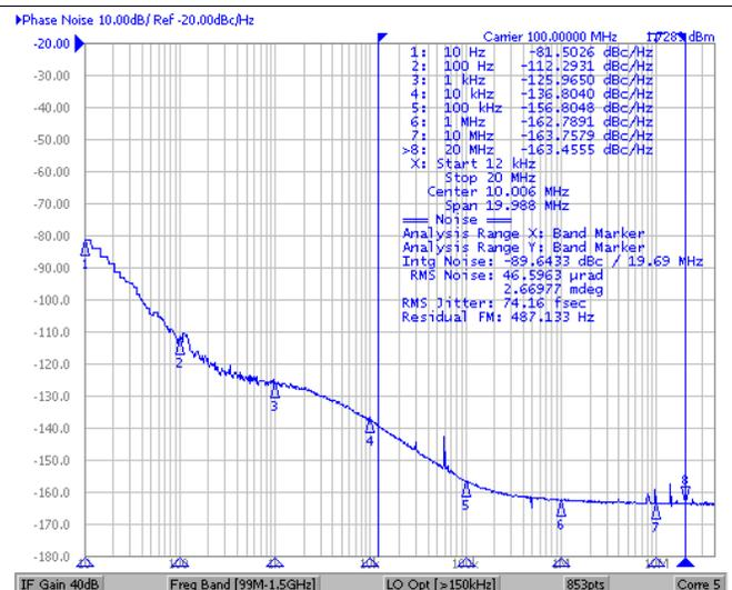
Jitter = 74 fs RMS (12 kHz to 20 MHz)
