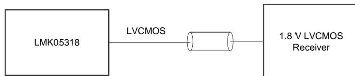
Figure 47. 1.8-V LVCMOS Output to 1.8-V LVCMOS Receiver
