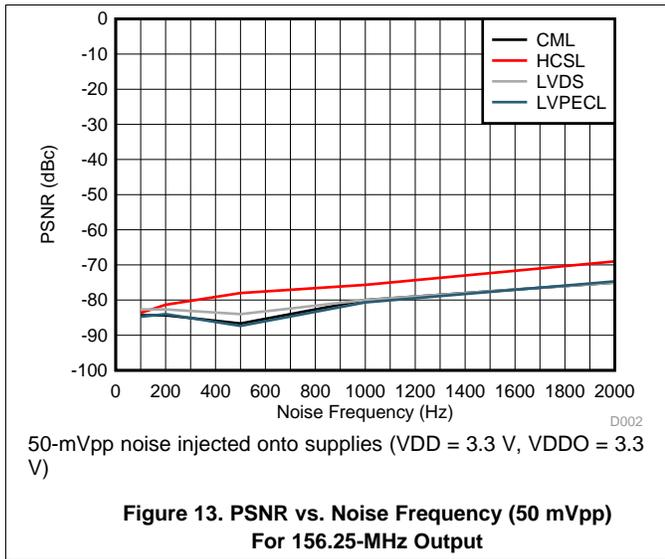
Figure 13. PSNR vs. Noise Frequency (50 mVpp) For 156.25-MHz Output
