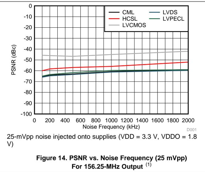
Figure 14. PSNR vs. Noise Frequency (25 mVpp) For 156.25-MHz Output (1)
