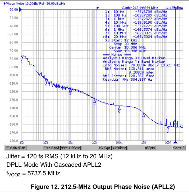
Figure 12. 212.5-MHz Output Phase Noise (APLL2)
