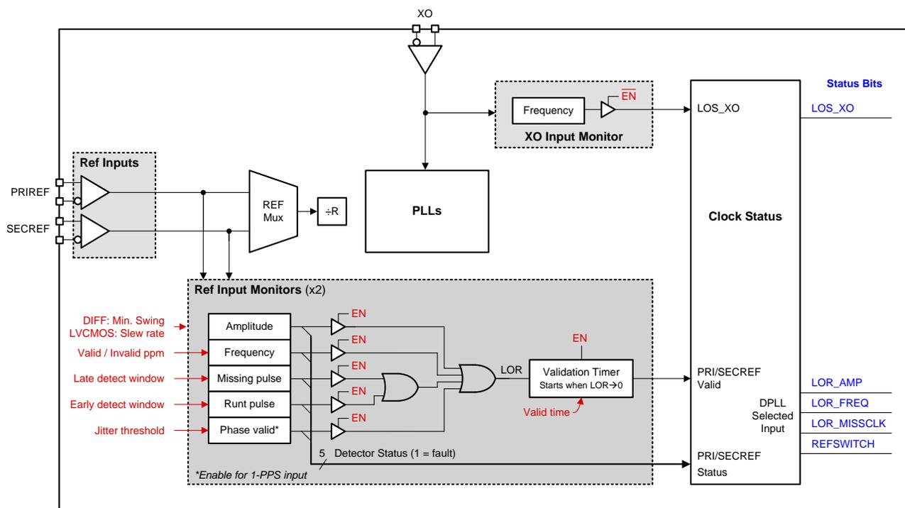
Figure 37. Clock Monitors for Reference and XO Inputs
