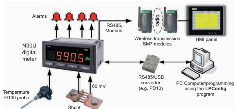
Measurement and visualization of analog standard signals: Pt100, TC, 20 mA, 60 mV, 10 V. Measured parameters are transmitted to the HMI operator panel through radio modules.
