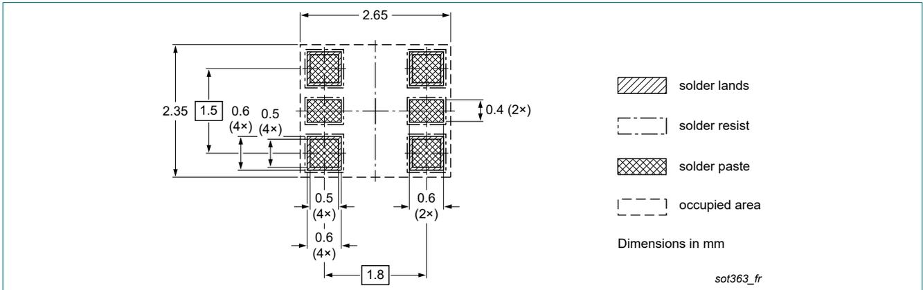
Fig. 12. Reflow soldering footprint for TSSOP6 (SOT363)
