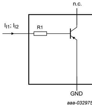
Fig. 10. Resistor test circuit
