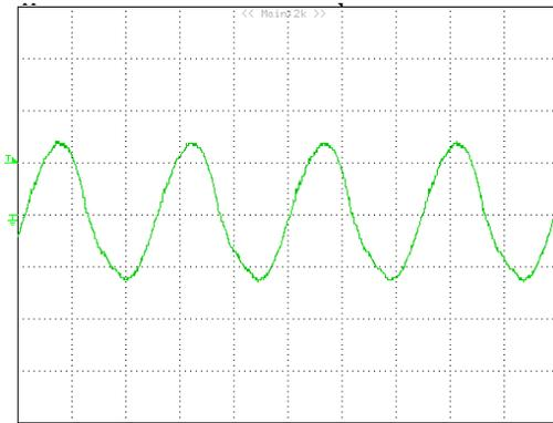
**Figure 10:** Input Terminal Ripple Current,  $i_c$ , at full rated output current and nominal input voltage with 12  $\mu H$  source impedance and 33  $\mu F$  electrolytic capacitor (200 mA/div, 1  $\mu s$ /div)
