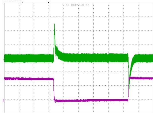
**Figure 8.2:** Output voltage response to step-change in load current 0A-3.2A-0A, max;  $di/dt = 2.5A/\mu s$ ). Load cap:  $10\mu F$  tantalum capacitor and  $1\mu F$  ceramic capacitor. Top Trace: Vout (0.2V/div, 200us/div), Bottom Trace: Iout (2A/div). Scope measurement should be made using a BNC cable (length shorter than 20 inches). Position the load between 51 mm to 76 mm (2 inches to 3 inches) from the module
