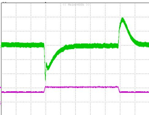
**Figure 8.1:** Output voltage response to step-change in load current (75%-50%-75% of  $I_{o,max}$ ;  $di/dt = 0.1A/\mu s$ ). Load cap:  $10\mu F$  tantalum capacitor and  $1\mu F$  ceramic capacitor. Top Trace: Vout (0.15V/div, 200us/div), Bottom Trace: Iout (5A/div). Scope measurement should be made using a BNC cable (length shorter than 20 inches). Position the load between 51 mm to 76 mm (2 inches to 3 inches) from the module
