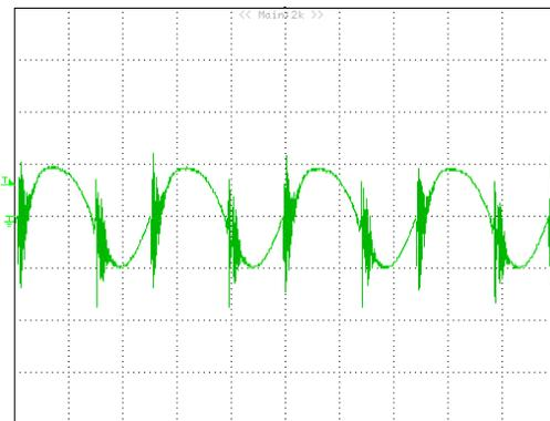
**Figure 13:** Output voltage ripple at nominal input voltage and rated load current ( $I_o=7.5A$ ) (50 mV/div, 1  $\mu s$ /div)
