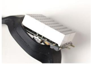
Place the clear back first into the band so it's at the bottom. Then stretch the band and scootch the assembly in, pulling the rubber to fit around!
