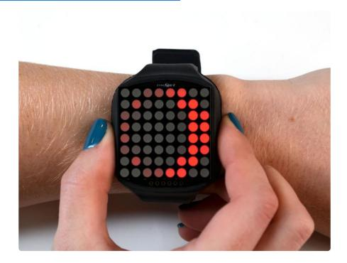
Engineered for greatness by PaintYourDragon, this watch squeezes over 1000 full time displays out of a coin battery, and a 1+ year 'resting' lifetime, so you can use this as a day-to-day time keeper.
