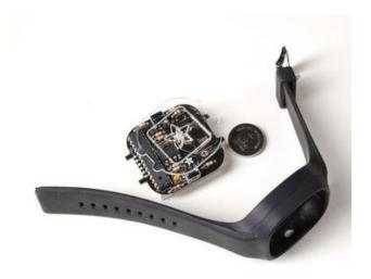
Get the remaining parts out of the kit - a 20mm coin battery, silicone band and optional clear plastic back
