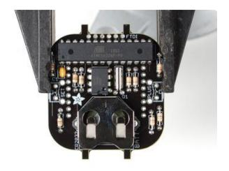
Next we'll place both the battery holder, and the timing crystal. The battery of course is how we power the watch, and this holder keeps it in place. The timing crystal is the "Quartz Crystal" in watches, that keeps time by resonating
