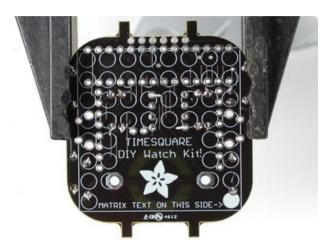
Next up we will put in the first chip. This chip has 8 legs and has the label DS1337 on top. Make sure you've got the right label on the chip.
