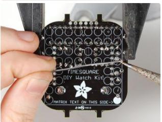
Important! Once you solder the matrix to the board, it is nearly impossible to diagnose or repair any soldering problems. If you have any doubts at all about your solder joints, post some clear photos to the forum now so our engineers can check it over.
