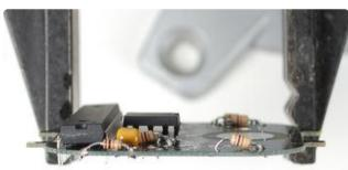
Next we'll do the big microcontroller chip. This chip is the brains, it does all of the displaying and button handling. Most of the time its 'sleeping' and when you press a button it wakes up and shows the time. It has a lot of pins because the matrix requires 16 pins to draw, and then you need some more pins for buttons, the RTC chip, reprogramming, etc.
