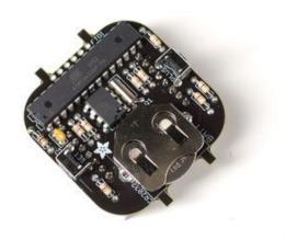
Insert a 20mm (CR2032) coin cell battery so that the flat + side is facing up and the bumpy side is facing down into the PCB
