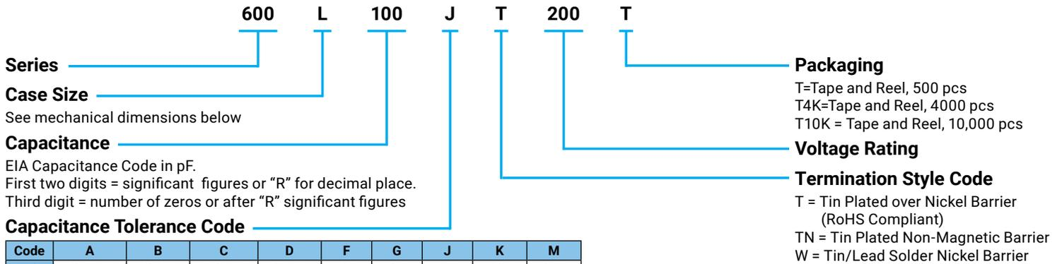
\*All Tape and Reel Packaging comes on 7" reels. The above part number refers to a 600L Series (case size L) 11 pF capacitor, J tolerance (±5%), 200 WVDC, with T termination (Tin Plated over Nickel Barrier, RoHS Compliant), Tape and Reel packaging.
