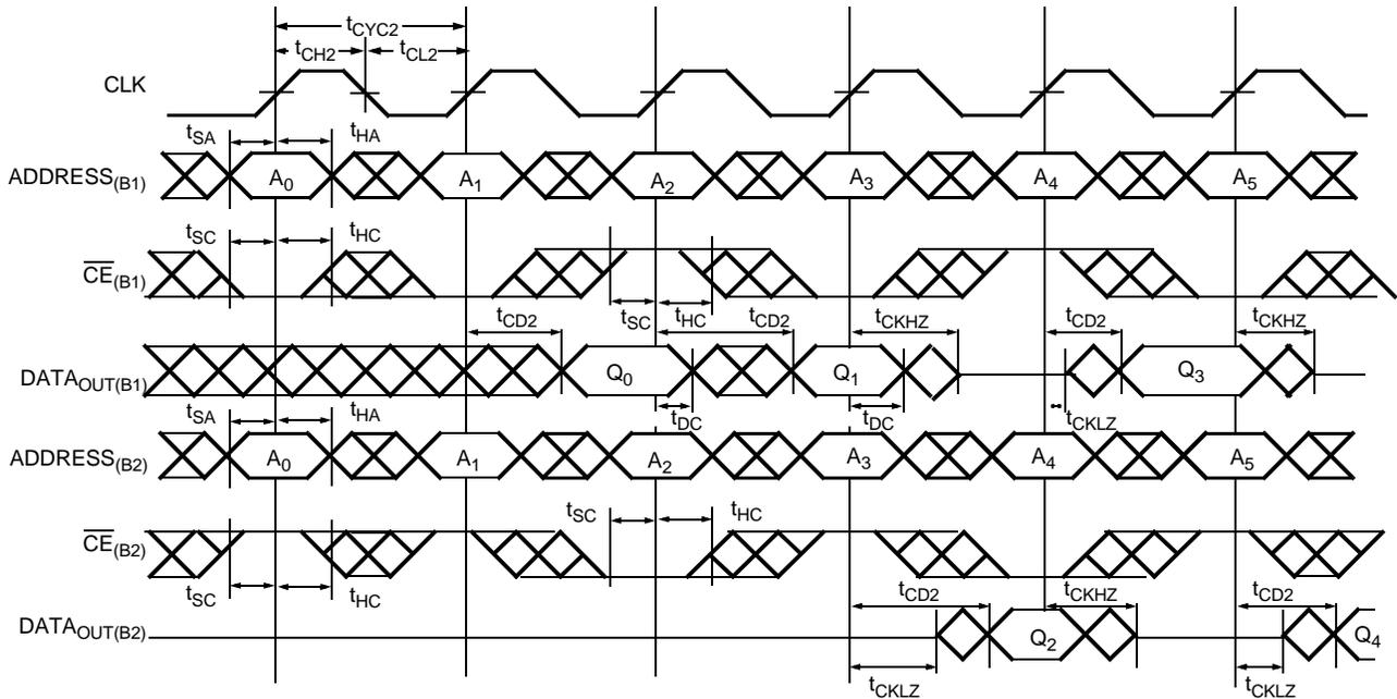
Figure 11. Read-to-Write-to-Read ( $\overline{OE} = \text{LOW}$ ) [36, 39, 40, 41, 42]
