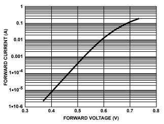
FIGURE 14. BOOTSTRAP DIODE I-V CHARACTERISTICS
