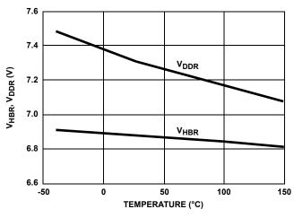
FIGURE 9. UNDERVOLTAGE LOCKOUT THRESHOLD vs TEMPERATURE
