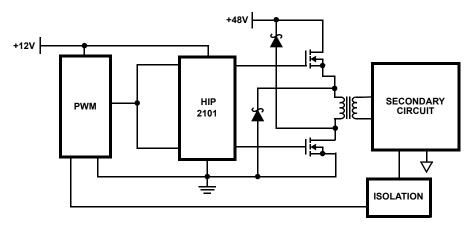
FIGURE 1. TWO-SWITCH FORWARD CONVERTER
