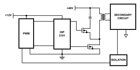
FIGURE 2. FORWARD CONVERTER WITH AN ACTIVE CLAMP
