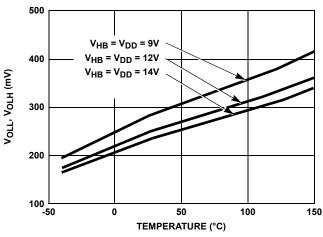
FIGURE 8. LOW LEVEL OUTPUT VOLTAGE vs TEMPERATURE
