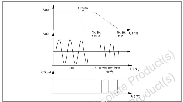
Figure 21. Thermal Foldback Diagram
