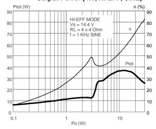
Figure 14. Power Dissipation vs. Average Ouput Power (Audio Program Simulation,  $4\Omega$ )
