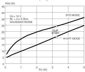
Figure 15. Power Dissipation vs. Average Ouput Power (Audio Program Simulation,  $2\Omega$ )
