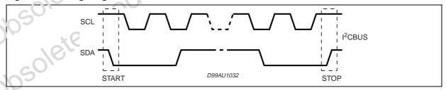
Figure 24. Acknowledge on the I<sup>2</sup>CBUS
