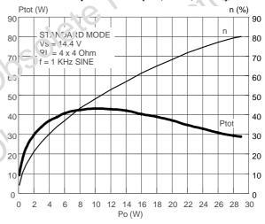
Figure 13. Power Dissipation & Efficiency vs.
