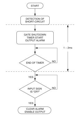
NOTE: Output voltage with protection circuit operating is about -IV\_EEI + 2V
