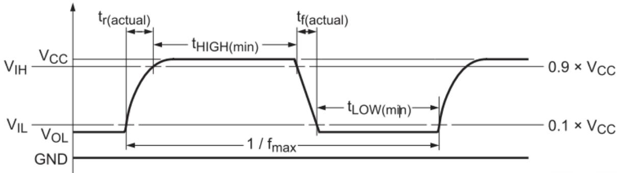
The rise and fall times are dependent upon translation voltages, the drive strength, the total node capacitance (CL) and the pull-up resistors (RPU) that are present on the bus. The node capacitance is the addition of the PCB trace capacitance and the device capacitance that exists on the bus.
