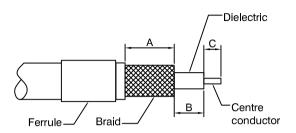
2) Tin the centre conductor of the cable. Insert the cable into the body. Make sure the braid is on the outside of the mandrel and the centre conductor is located in the mounting post.
