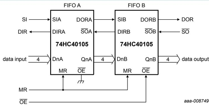
The 74HC40105 is easily cascaded to increase word capacity without external circuitry. In cascaded format, the FIFOs handle all necessary communications. Fig. 18 and Fig. 20 demonstrate the communication timing between FIFO A and FIFO B. Fig. 23 provides an overview of pulses and timing of two cascaded FIFOs, when shifted full and shifted empty again.
