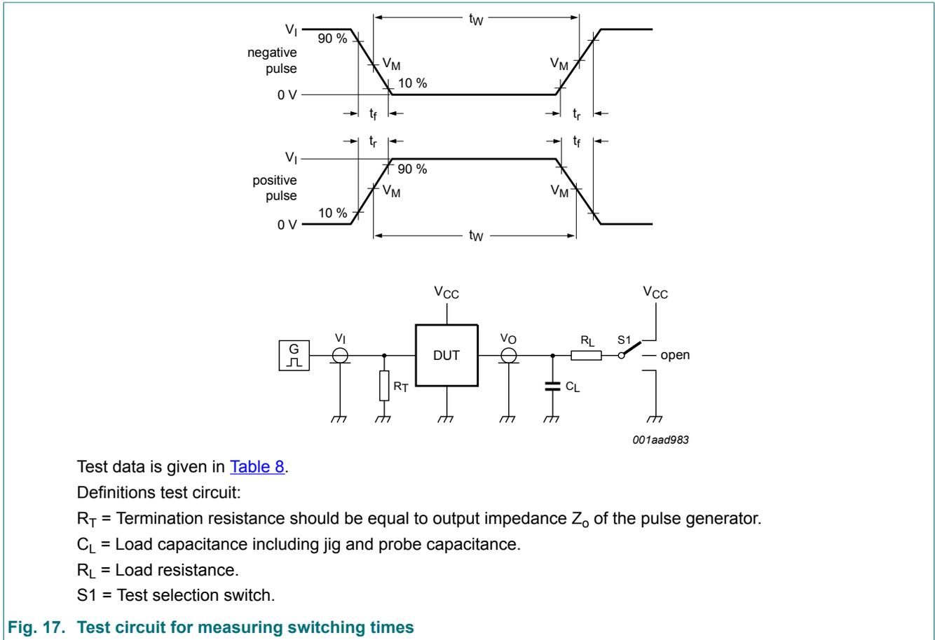
Fig. 17. Test circuit for measuring switching times
