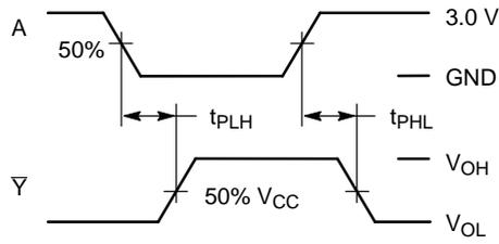
**Figure 4. Switching Waveforms**
