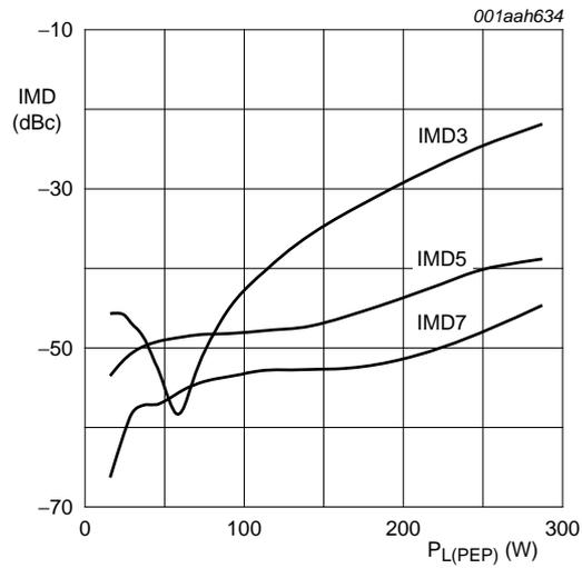
V<sub>DS</sub> = 32 V; I<sub>Dq</sub> = 1600 mA; f<sub>1</sub> = 2170 MHz; f<sub>2</sub> = 2170.1 MHz.
