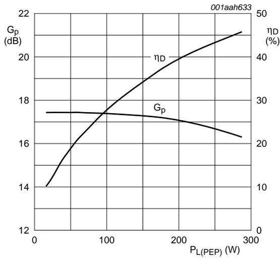
V<sub>DS</sub> = 32 V; I<sub>Dq</sub> = 1600 mA; f<sub>1</sub> = 2170 MHz; f<sub>2</sub> = 2170.1 MHz.
