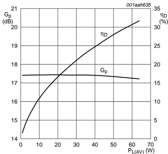
V<sub>DS</sub> = 32 V; I<sub>Dq</sub> = 1600 mA; f<sub>1</sub> = 2162.5 MHz; f<sub>2</sub> = 2167.5 MHz; carrier spacing 5 MHz.
