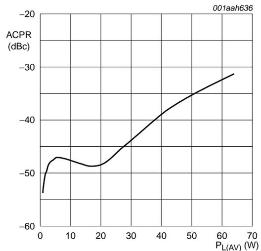
V<sub>DS</sub> = 32 V; I<sub>Dq</sub> = 1600 mA; f<sub>1</sub> = 2162.5 MHz; f<sub>2</sub> = 2167.5 MHz; carrier spacing 5 MHz.
