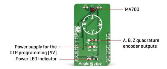
The magnetic field is only sensed along the horizontal (XZ) plane by utilizing an array of aligned Hall sensors. This allows sampling of the absolute angular position of a diametrically magnetized cylinder, typically attached at the end of the rotor shaft. Unlike
