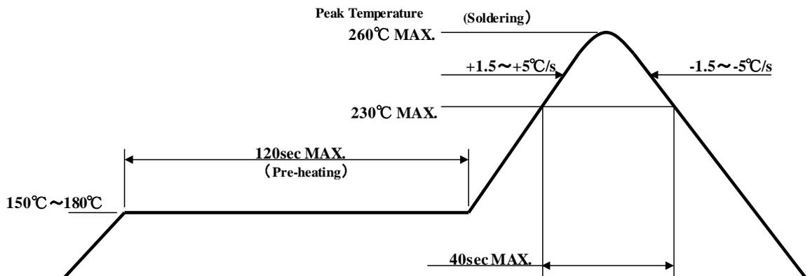
Note 1 Temperature Profile for the reflow should be set to the surface temperature of resin which is on the top of LED. This should be the maximum temperature for soldering. Lowering the heating temperature and decreasing heating time is very effective in achieving higher reliability.
