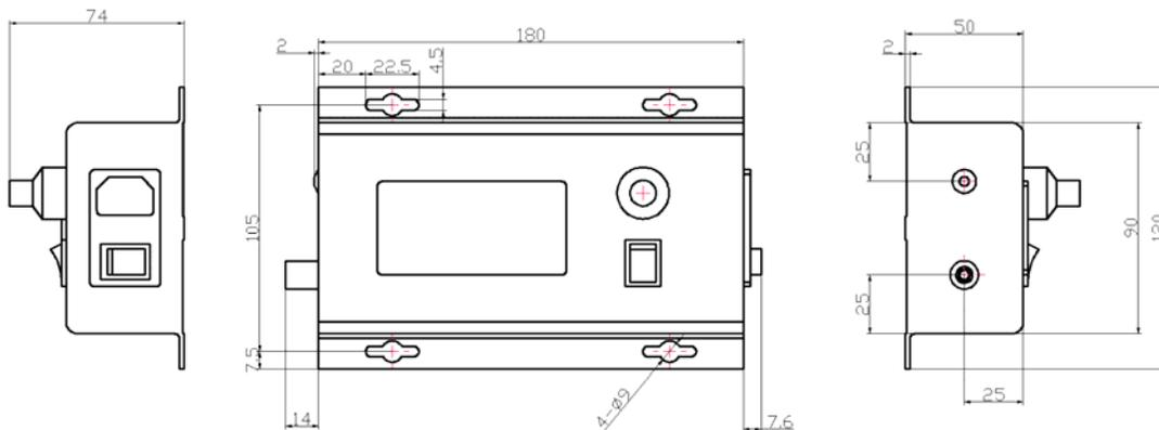
Figure 9. Dimensions for AHVACN15KV1MABT
