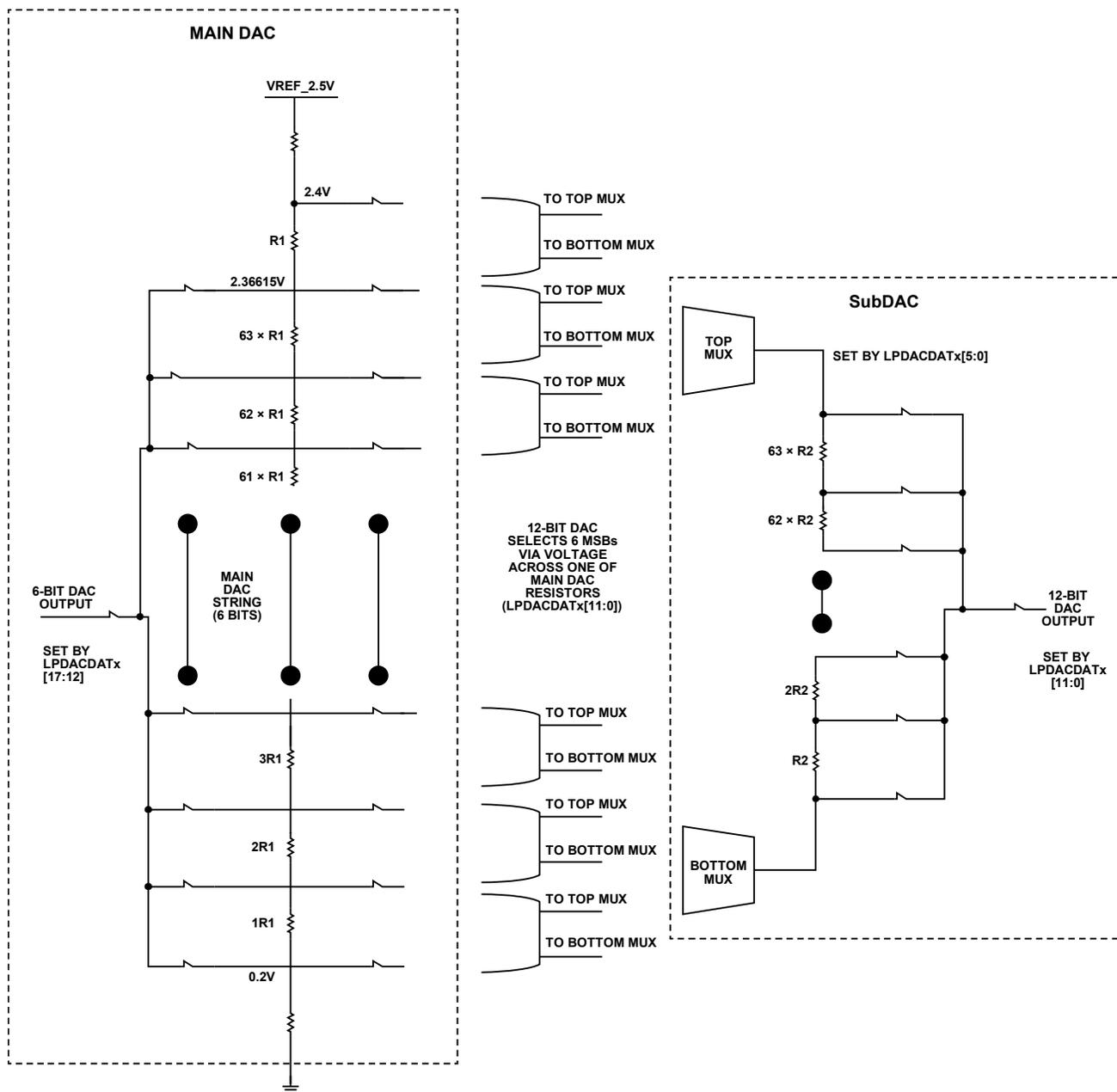
Figure 19. Block Diagram of Low Power DACs
