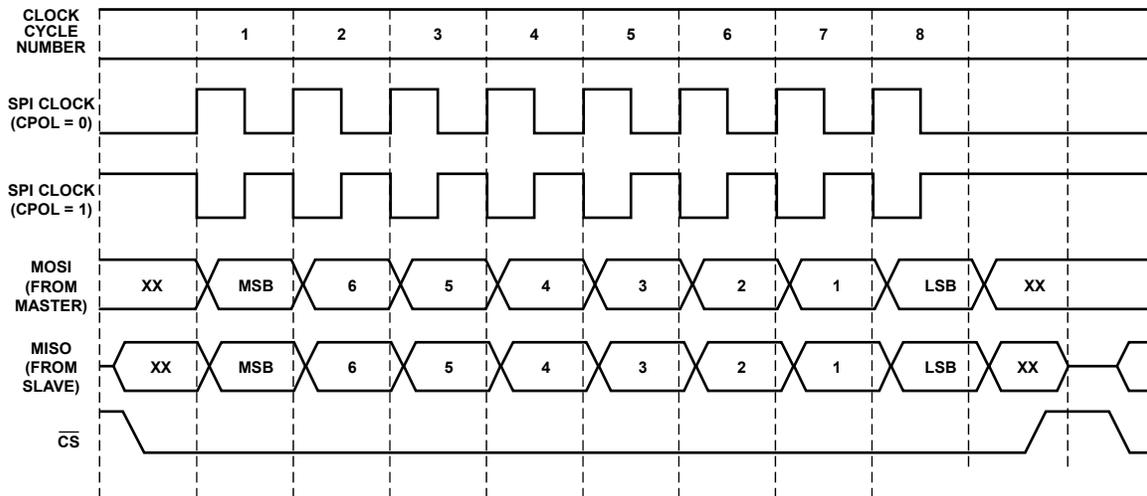
Figure 62. SPI Transfer Protocol, CPHA = 1
