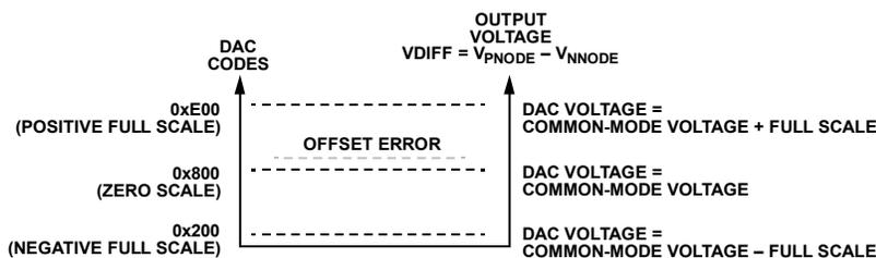
Figure 25. High Speed DAC Transfer Function
