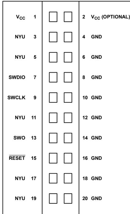
Figure 68. SWD 20-Pin Connector Pinout
