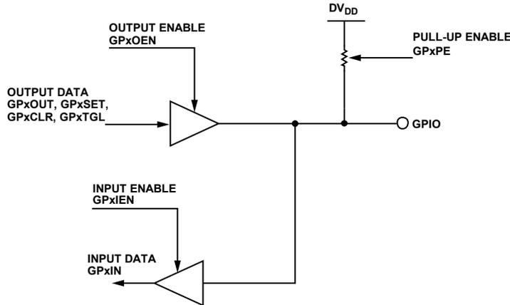
Figure 55. GPIO Structure for Pins with Pull-Up Resistors
