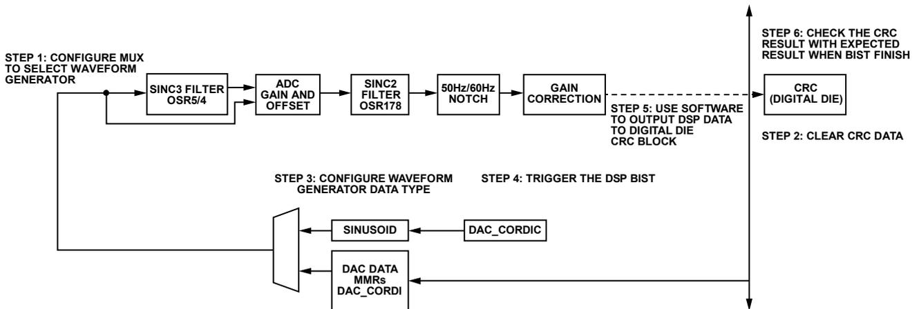
Figure 13. ADC Built In Self Test Feature
