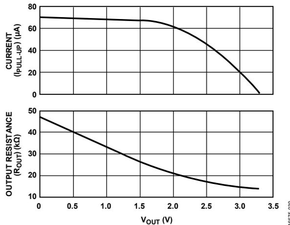
Figure 56. Typical Port 0, Port 1, and Port 2 Pull-Up Characteristics
