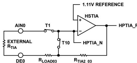
Figure 22. Connecting External  $R_{TIA}$  Across the High Speed TIA
