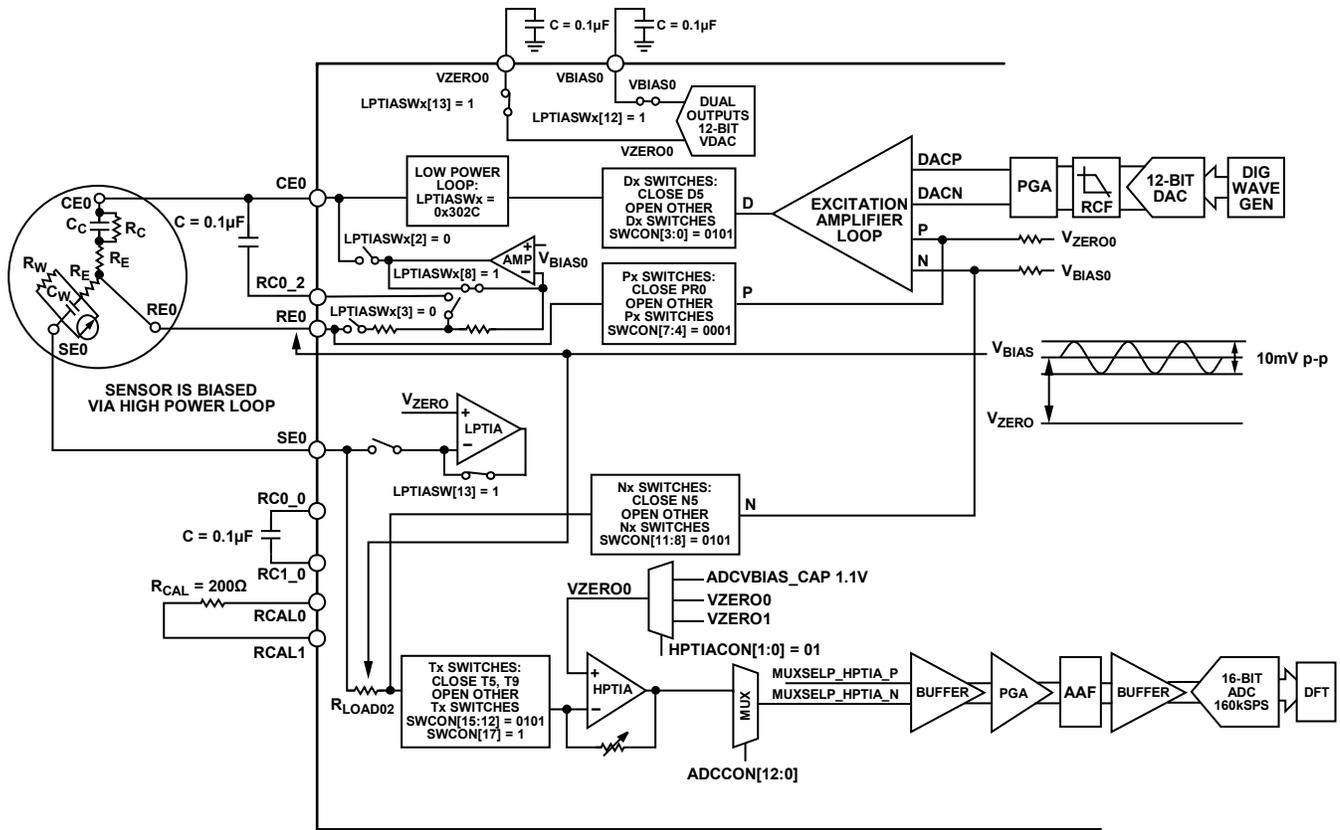
Figure 42.  $R_{LOAD02}$  Measurement
