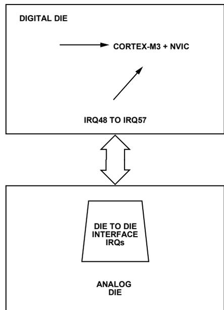
Figure 5. Analog Die Interrupt Connections to Digital Die
