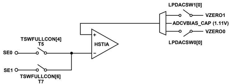
Figure 17. Low Power TIA, Low Power Potentiostat, and Low Power DAC Switches for Channel 1
