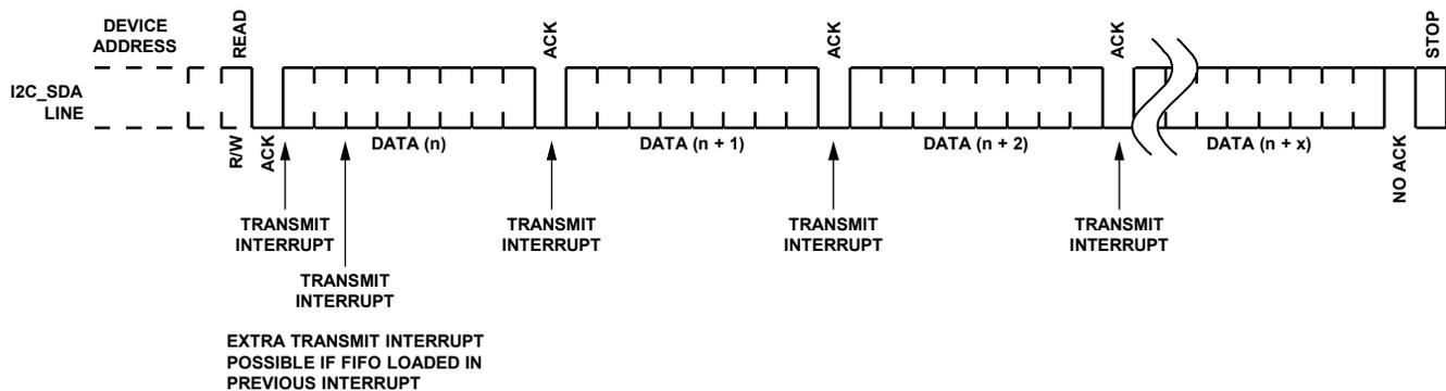
Figure 60. I<sup>2</sup>C Slave Transmit Interrupt Details
