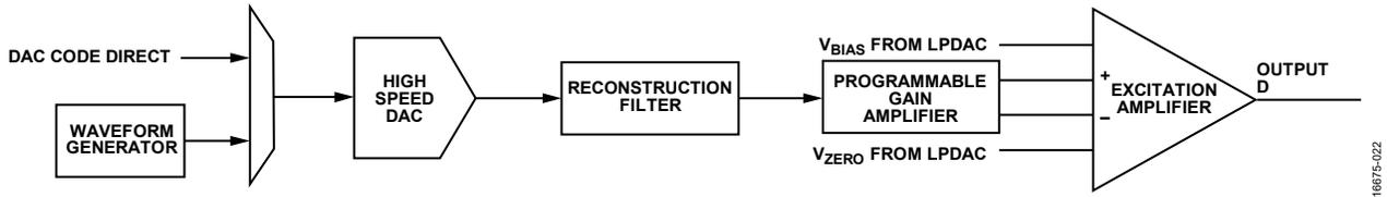
Figure 23. Overview of High Speed DAC Blocks
