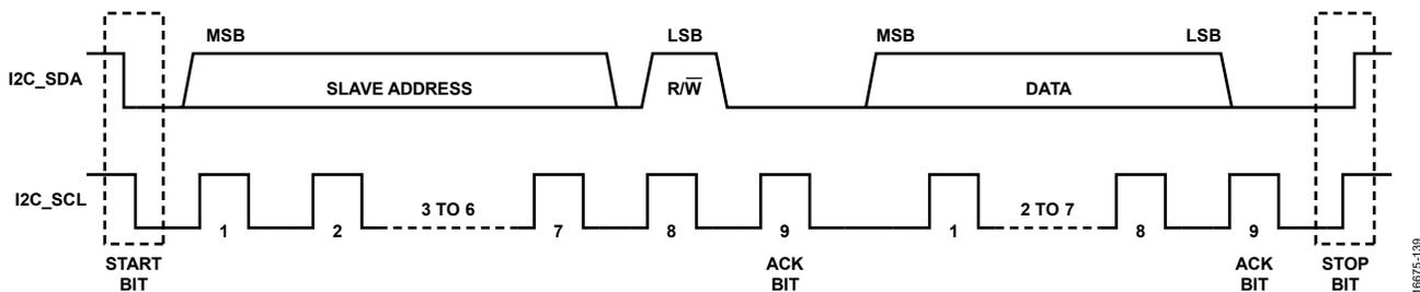
Figure 57. Typical I<sup>2</sup>C Transfer Sequence
