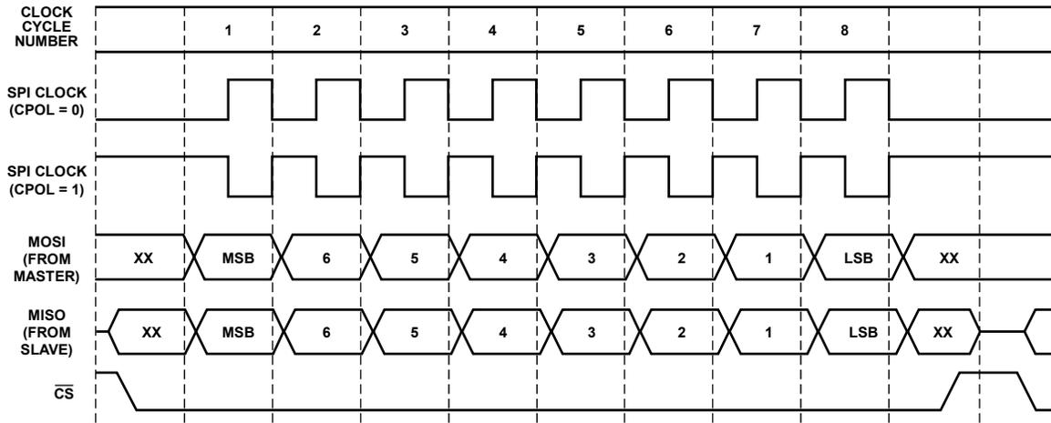
Figure 61. SPI Transfer Protocol, CPHA = 0
