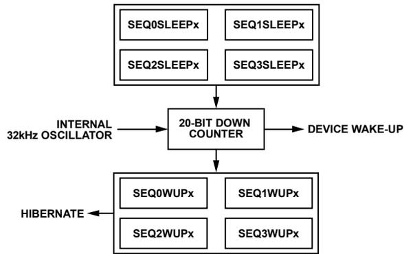
Figure 34. Sleep and Wake-Up Timer Block Diagram
