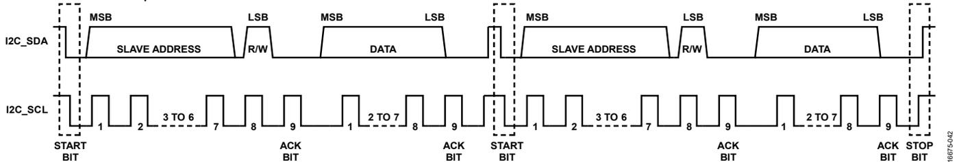
Figure 59. I<sup>2</sup>C Repeated Start Sequence
