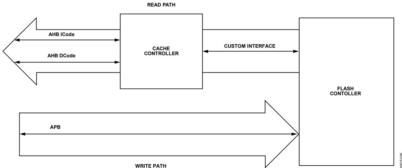
Figure 53. Flash Memory Read and Write Data Paths
