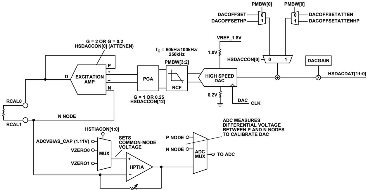
Figure 26. High Speed DAC Calibration Circuit Using  $R_{CAL}$
