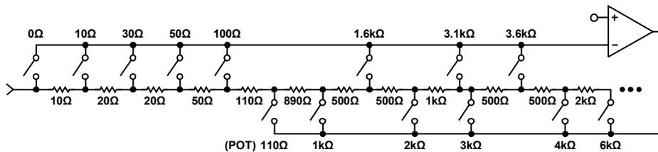
Figure 18. Low Power TIA  $R_{LOAD}$  and  $R_{GAIN}$  Configuration
