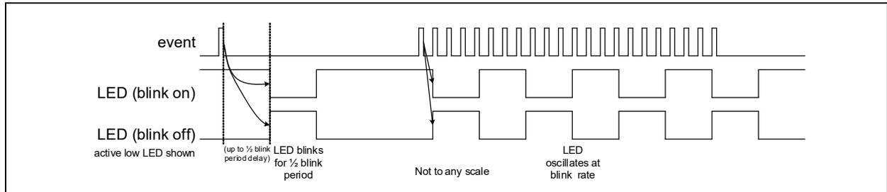
Pulse-stretch guarantees that an LED is asserted and de-asserted for a specific period of time when activity is either present or not present.
