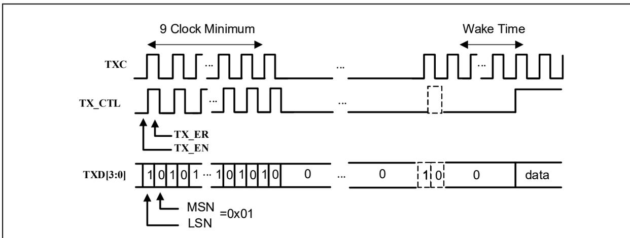
RGMII transmission at 100 Mbps from MAC-to-PHY uses both rising and falling edges of the **TXC** signal. The device uses the **TX\_CTL** pin to clock in the logical equivalent of the **TX\_EN** signal on the rising edge and the logical equivalent of the **TX\_ER** signal on the falling edge. It also uses the **TXD[3:0]** pins to clock in the TX data bits [3:0] on the rising edge.
