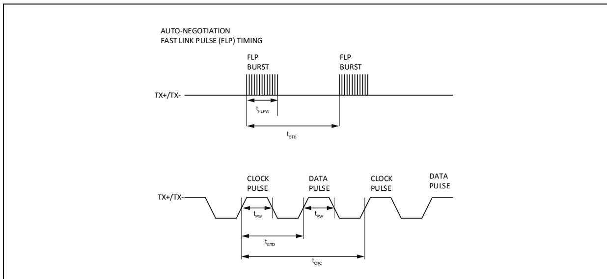
**TABLE 6-18: AUTO-NEGOTIATION FAST LINK PULSE (FLP) TIMING PARAMETERS**
