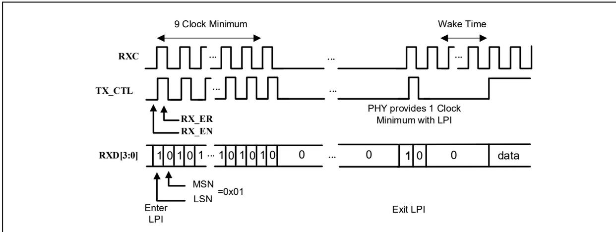
RGMII reception at 100 Mbps from PHY-to-MAC uses both rising and falling edges of the **RXC** signal. The device uses the **RX\_CTL** pin to clock out the logical equivalent of the **RX\_DV** signal on the rising edge and the logical equivalent of the **RX\_ER** signal on the falling edge. It also uses the **RXD[3:0]** pins to clock out the RX data bits [3:0] on the rising edge.
