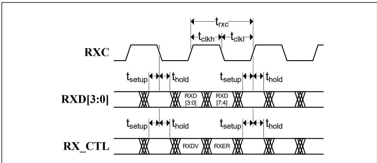
**TABLE 6-15: RGMII RXC INTERNAL DELAY ENABLED (RGMII ID MODE / TC6 DoS MODE) TIMING VALUES**
