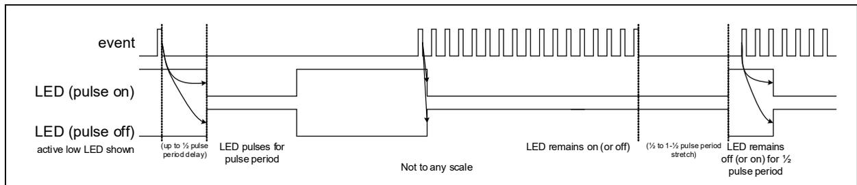
The blink / pulse stretch rate can be configured, as detailed in [Section 5.19.3.1.3, "Rate of LED Blink or Pulse-Stretch"](#).
