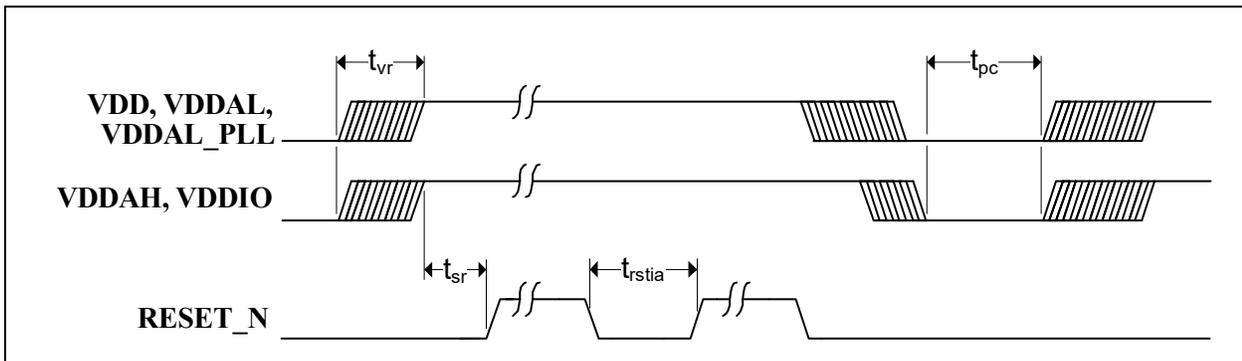
The recommended power-up sequence is to have the transceiver (VDDAH) and digital I/O (VDDIO) voltages power up before the 1.1V core (VDD, VDDAL, VDDAL\_PLL) voltage. If the 1.1V core must power up first, the maximum lead time for the 1.1V core voltage with respect to the transceiver and digital I/O voltages should be 200  $\mu$ s.
