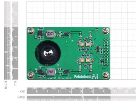
The OakSense H60Q is a camera kit based on the MLX75026 Time-of-Flight (ToF) sensor which is a complete camera for real-time visualization, recording, and analysis of data by emitting and receiving near-infrared light. The MLX75026 ToF sensor can be realized a very compact 3D Camera design based on the basic three-way low-voltage power supply architecture of sensor chip. In the case of the characteristic of the MLX75027 sensor, the kit contains an additional temperature sensor.
