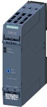
Thermistor motor protection relay Standard evaluation unit 22.5 mm enclosure Spring-type terminal 2 change-over contacts hard gold-plated US = 24 V-240 V AC/DC Manual/Auto/Remote reset with ATEX approval 2 LEDs (READY/TRIPPED) Safe galvanic isolation Test/reset button Wire break monitoring Short circuit monitoring non-volatile
