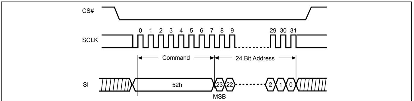
**Figure 35. Block Erase (BE) Sequence (Command D8)**
