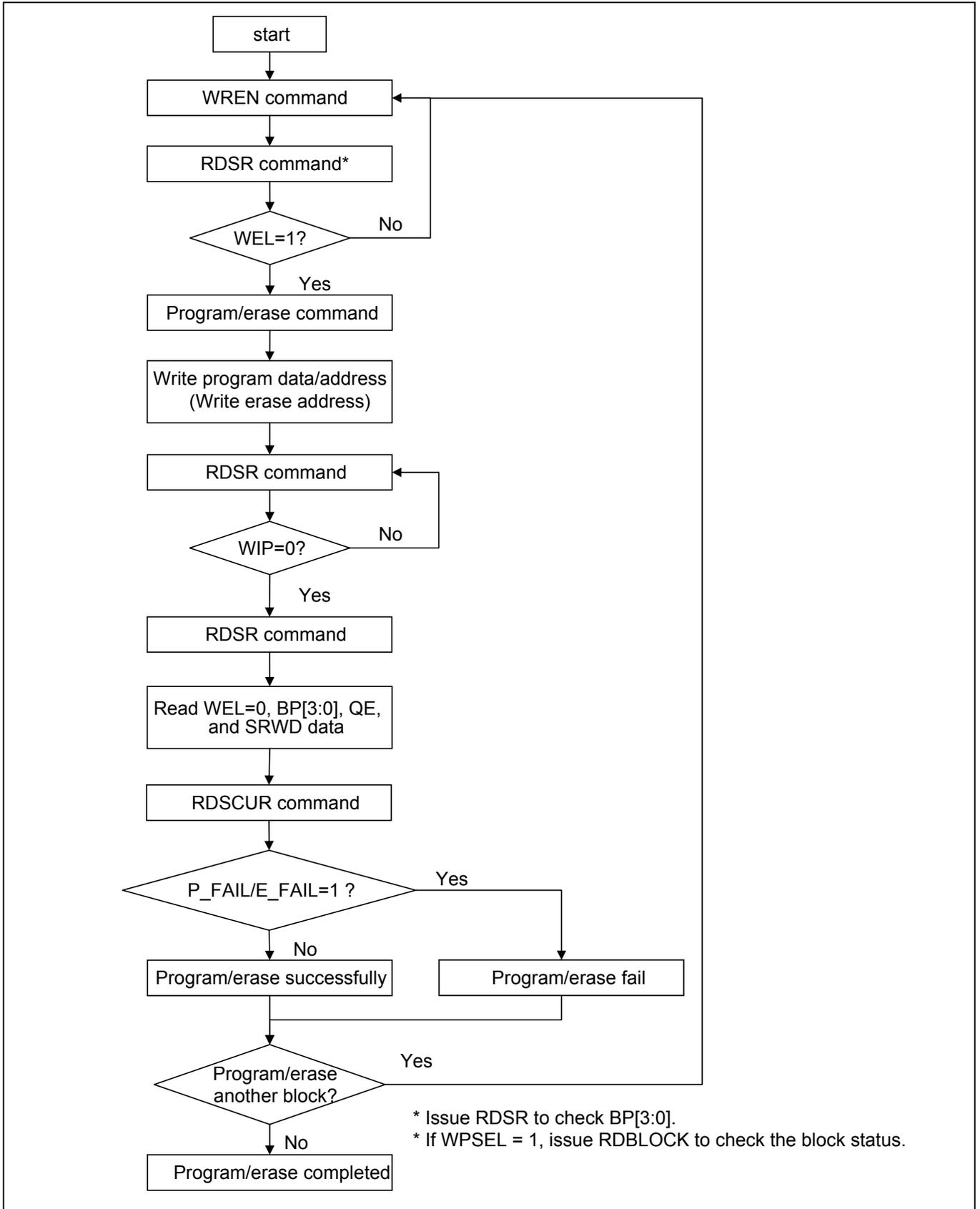
**Figure 5. WRSR Flow**
