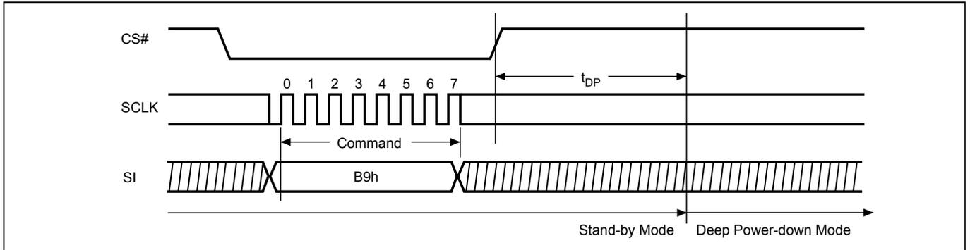
**Figure 38. Release from Deep Power-down and Read Electronic Signature (RES) (Command AB)**
