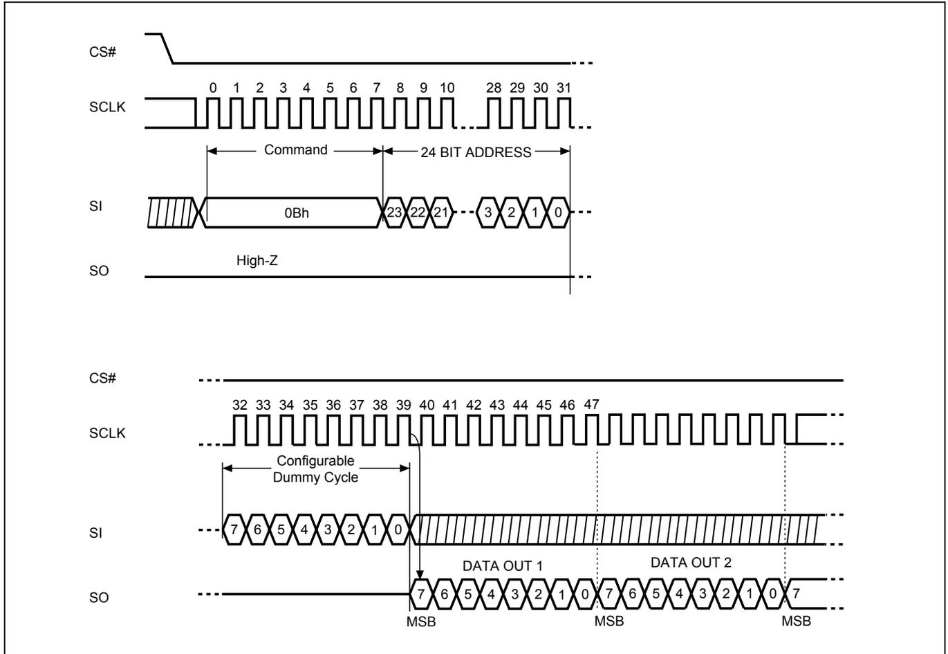
**Figure 26. Dual Read Mode Sequence (Command 3B)**
