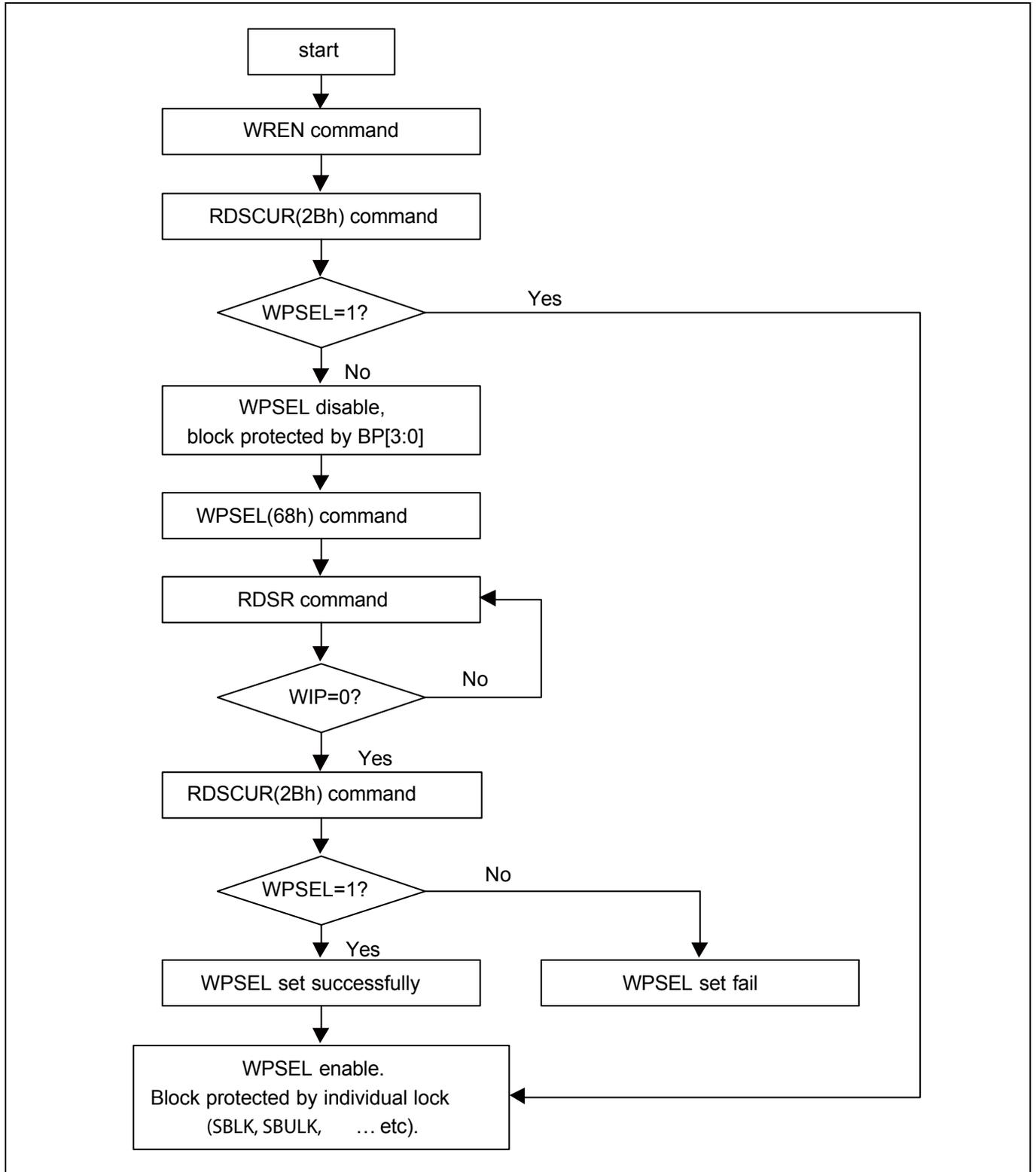
**10-26. Single Block Lock/Unlock Protection (SBLK/SBULK)**
