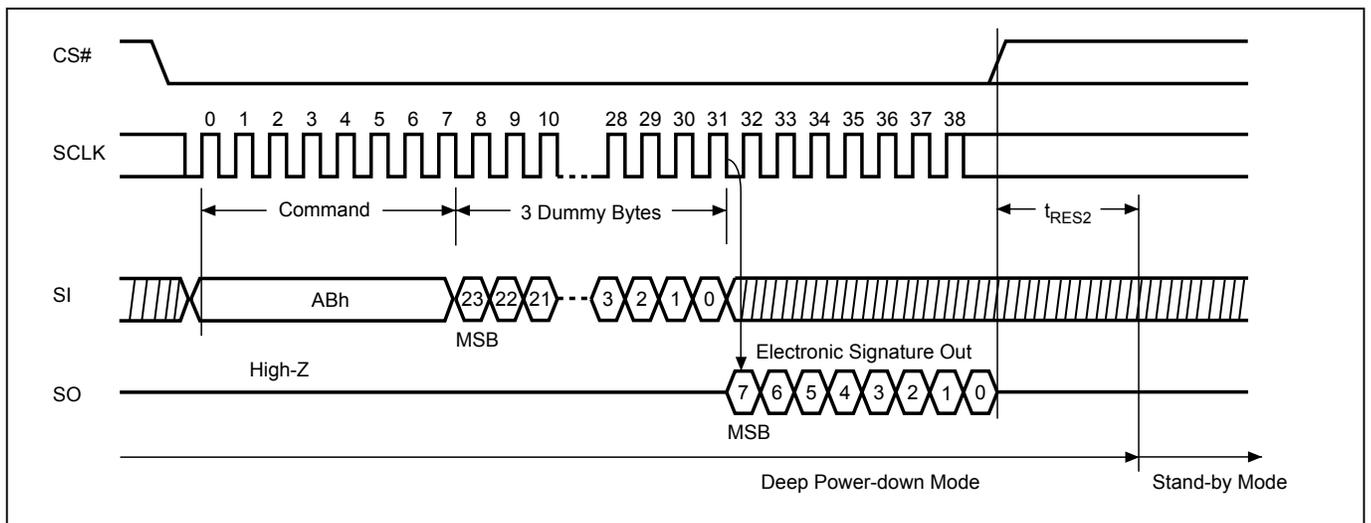
**Figure 39. Release from Deep Power-down (RDP) Sequence (Command AB)**
