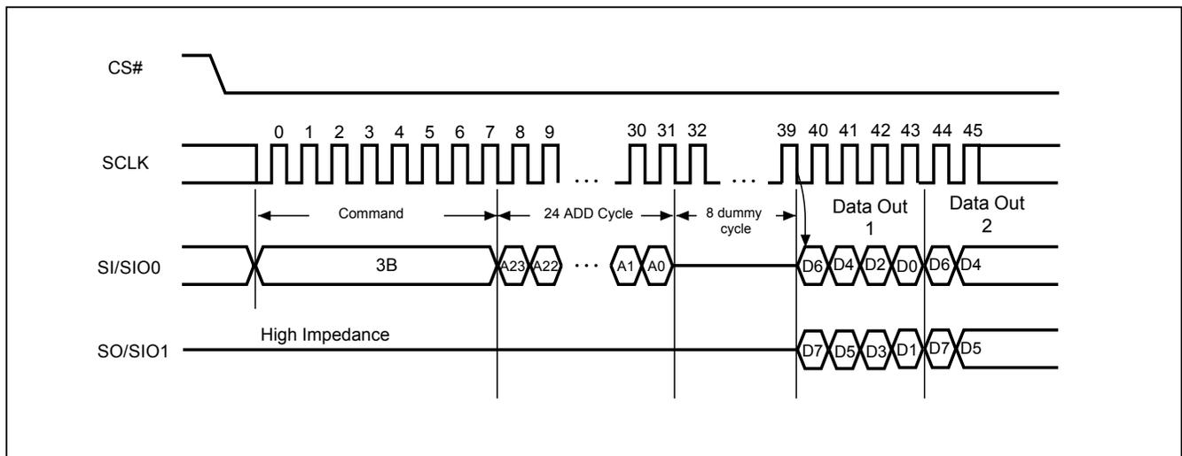
**Figure 27. 2 x I/O Read Mode Sequence (Command BB)**
