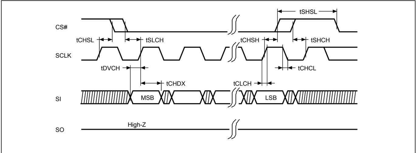
**Figure 16. Output Timing**
