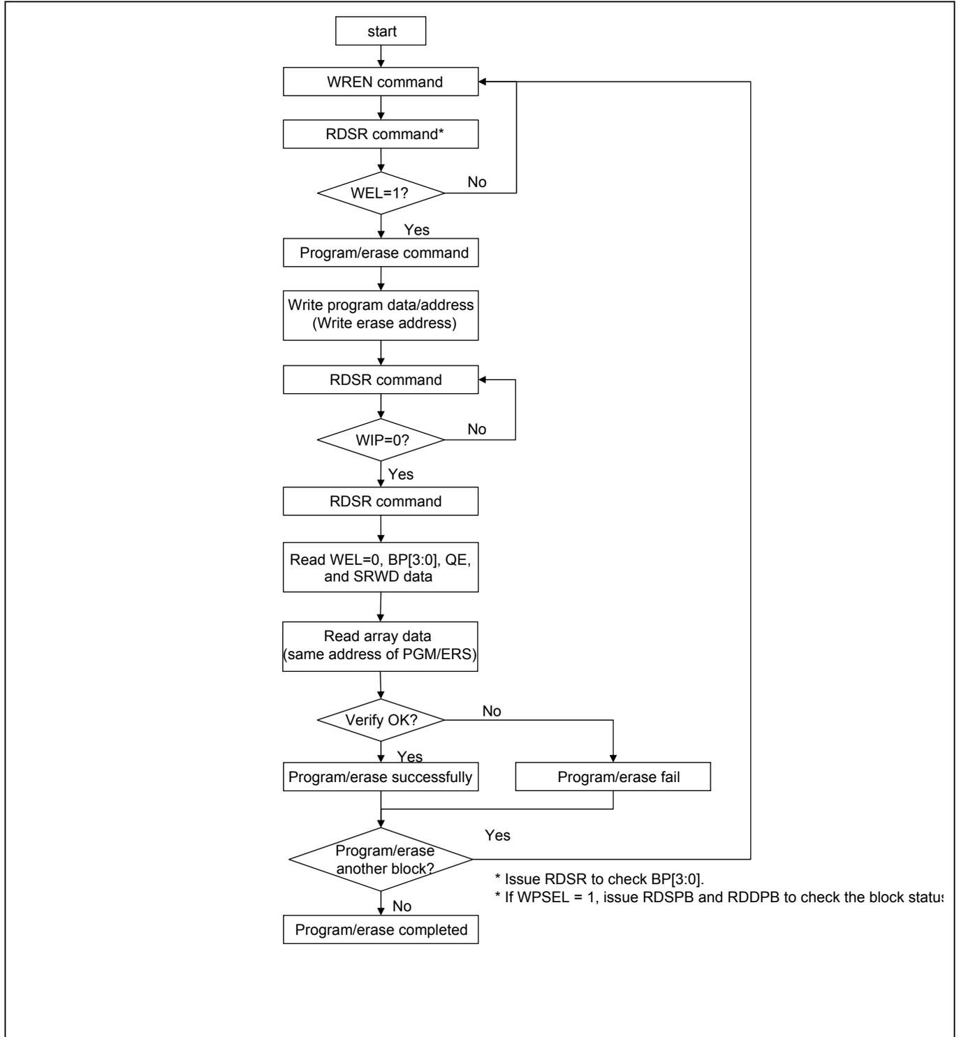
Figure 4. Program/ Erase Flow without Read Array Data (read P\_FAIL/E\_FAIL flag)
