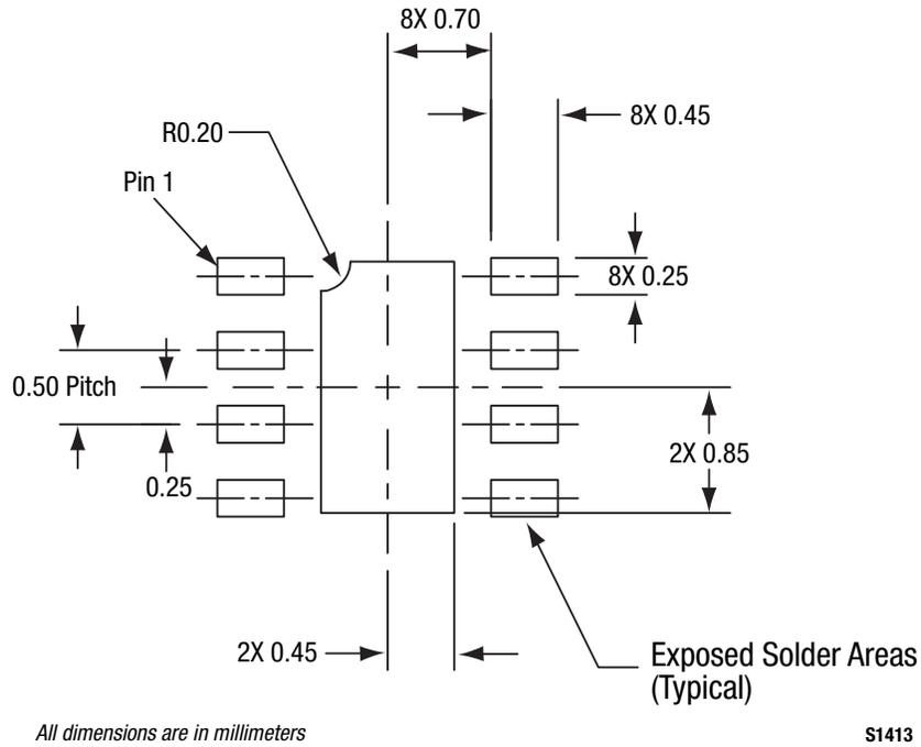
**Figure 29. SKY67014-396LF PCB Layout Footprint (Top View)**
