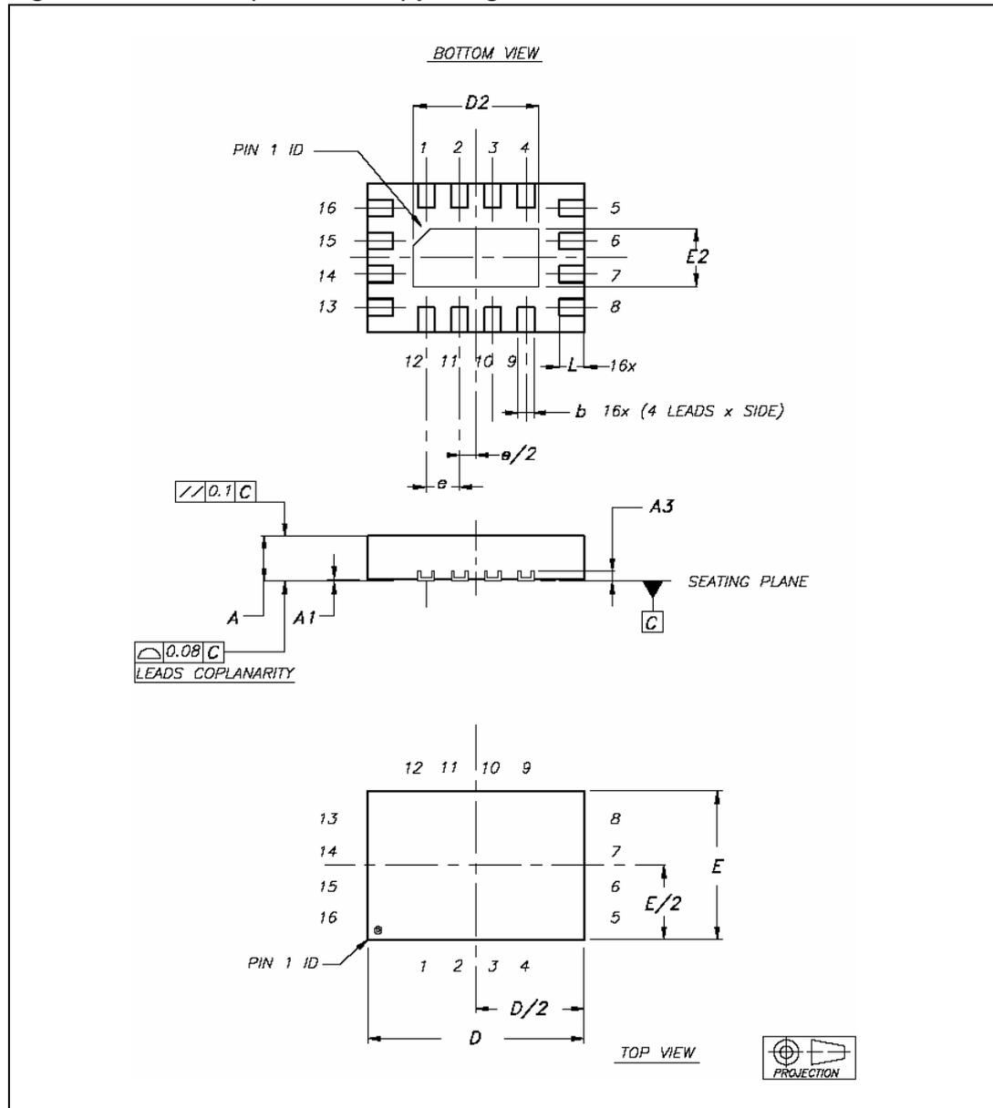
**Table 9. QFN16L (2.6 x 1.8 mm) mechanical data**
