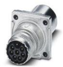
Panel feed-through, straight, SPEEDCON locking, M17, number of positions: 7+PE, type of contact: Pin, Crimp connection, Flat gasket,  $4x \varnothing 3.2$ , shielded: yes, flange dimensions: 25.75 mm x 25.75 mm, cable diameter range: 3.5 mm ... 5.5 mm
