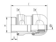
SKINTOP® HYGIENIC is a stainless steel cable gland that uses FDA-approved material and is designed with special features which prevent micro-organisms and bacteria from sticking to the surface. It has an IP68/69 rating and withstands high pressure and high temperature washdowns. SKINTOP® HYGIENIC-R includes a reducer bushing.
