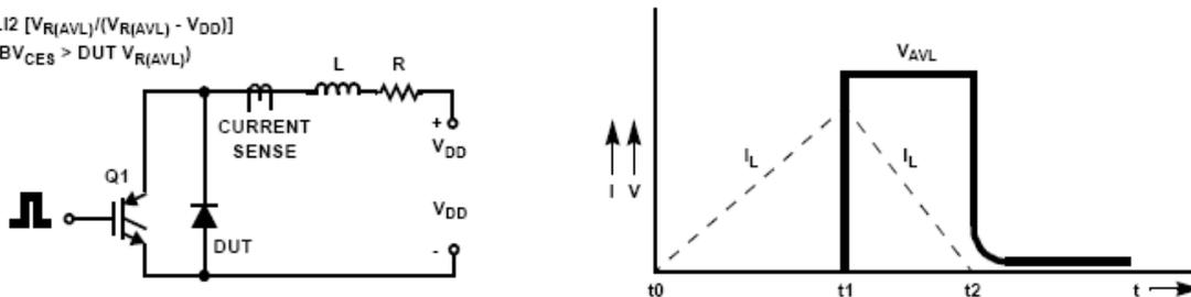
Figure 2. Unclamped Inductive Switching Test Circuit & Waveform
