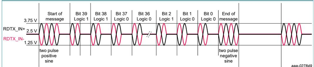
Figure 5. Transformer communication signaling
