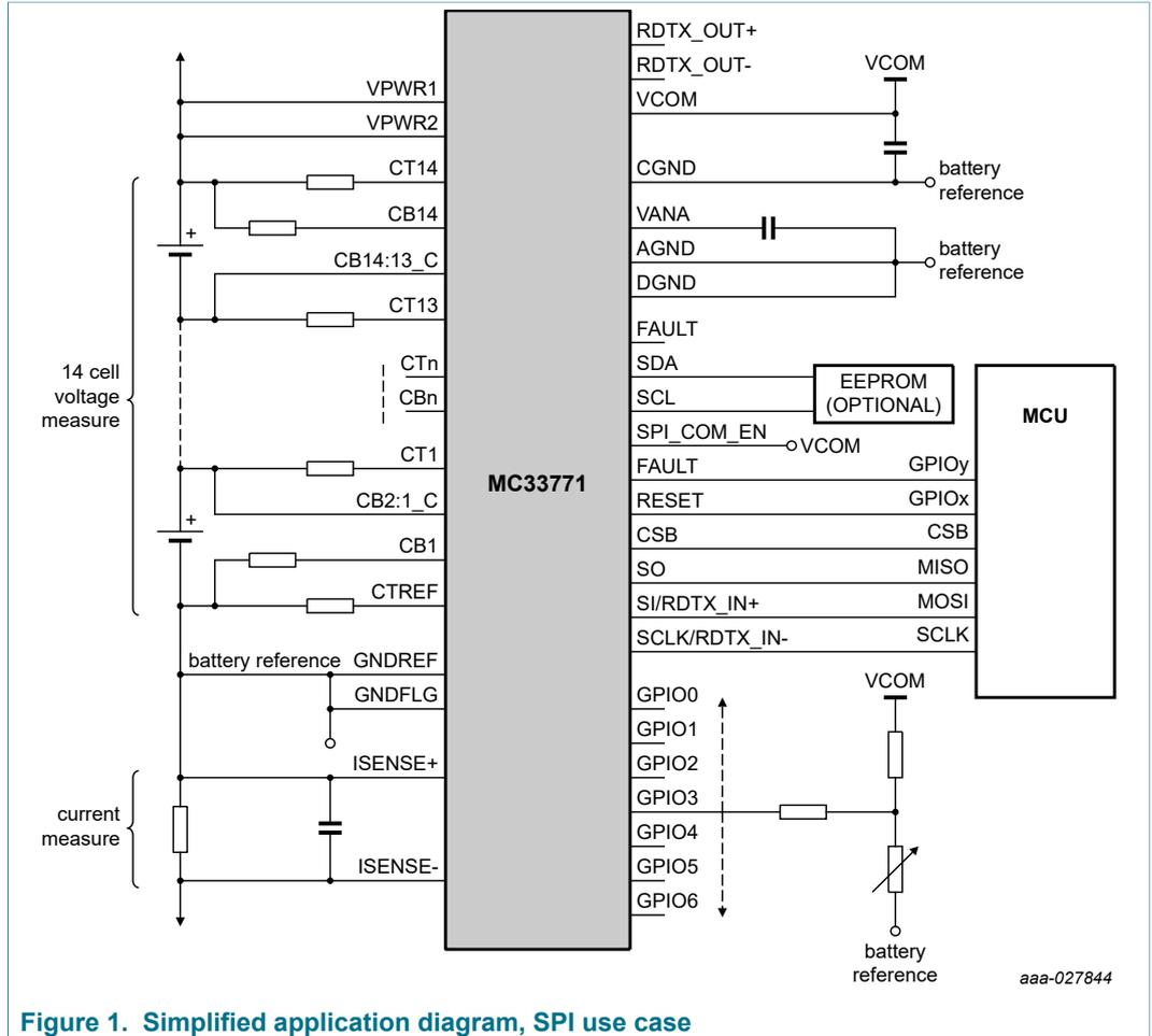
Figure 1. Simplified application diagram, SPI use case
