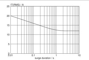
Fig.5. Maximum permissible repetitive rms on-state current  $I_{T(RMS)}$ , versus surge duration, for sinusoidal currents, f = 50 Hz;  $T_{hs} \le 56$  °C.
