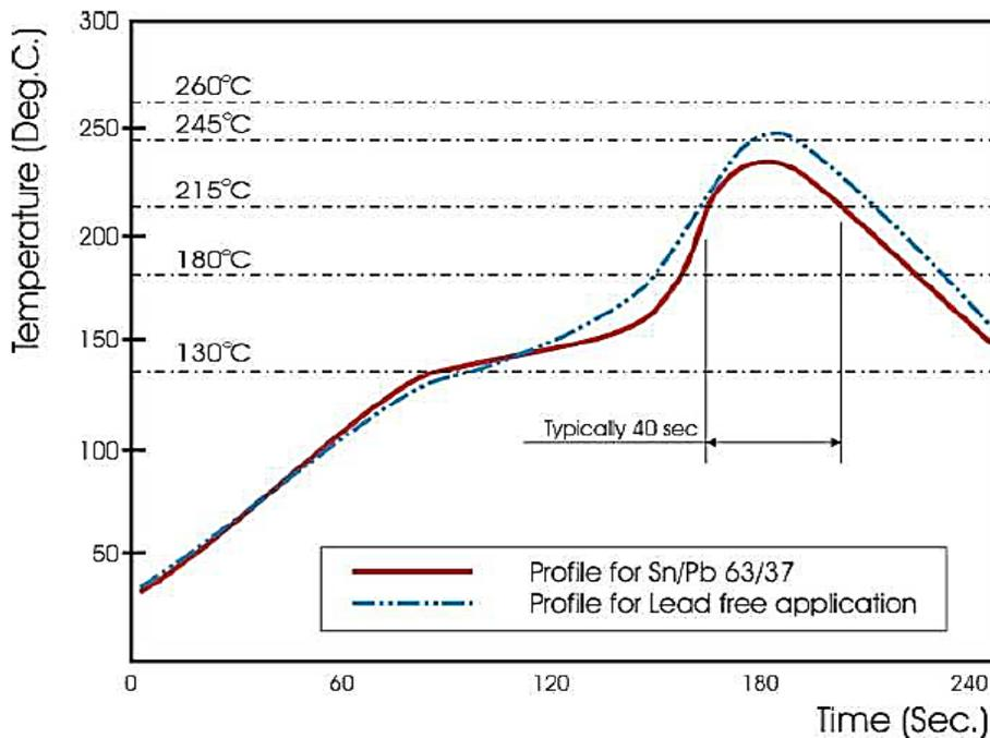
Fig 2. Infrared soldering profile for Chip Resistors
