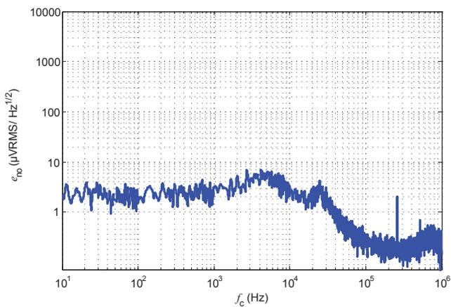
Figure 14: Output noise voltage spectral density
