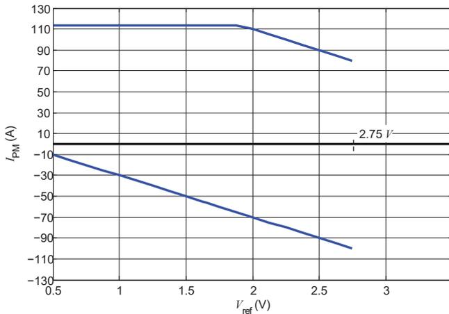
Figure 32: Measuring range versus external  $V_{ref}$  LESR 25-NP
