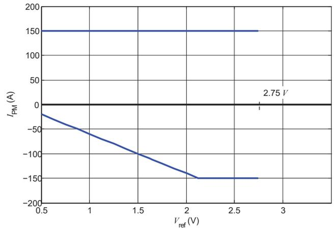
Figure 33: Measuring range versus external  $V_{ref}$  LESR 50-NP
