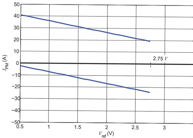
Figure 30: Measuring range versus external  $V_{ref}$  LESR 6-NP
