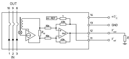
Figure 27: Test connection
