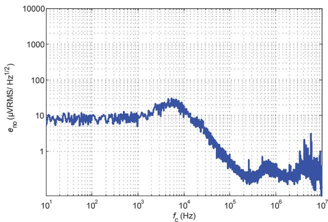
Figure 4: Output noise voltage spectral density
