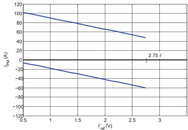
Figure 31: Measuring range versus external  $V_{ref}$  LESR 15-NP
