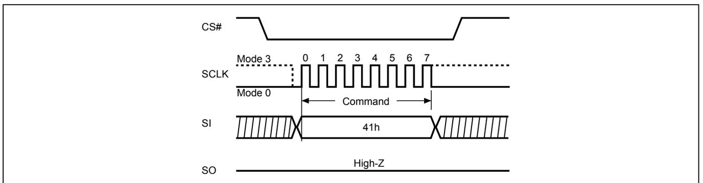
**Figure 12. Factory Mode Enable (FMEN) Sequence (QPI Mode)**
