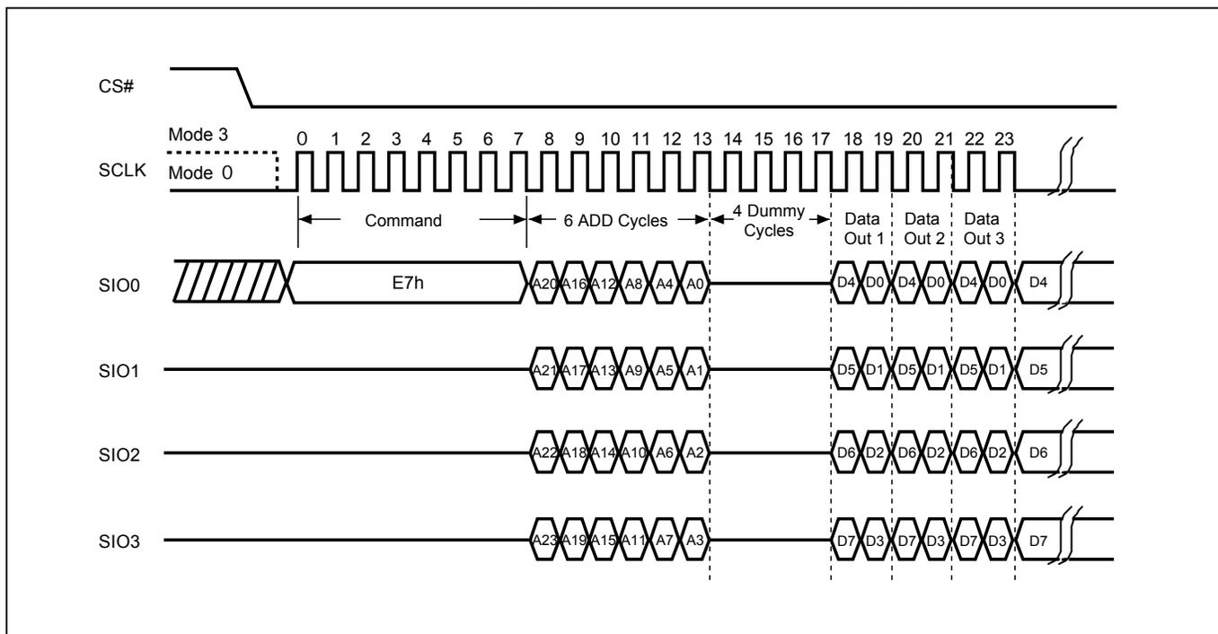
**Figure 32. 4 x I/O Read Mode Sequence (SPI Mode)**
