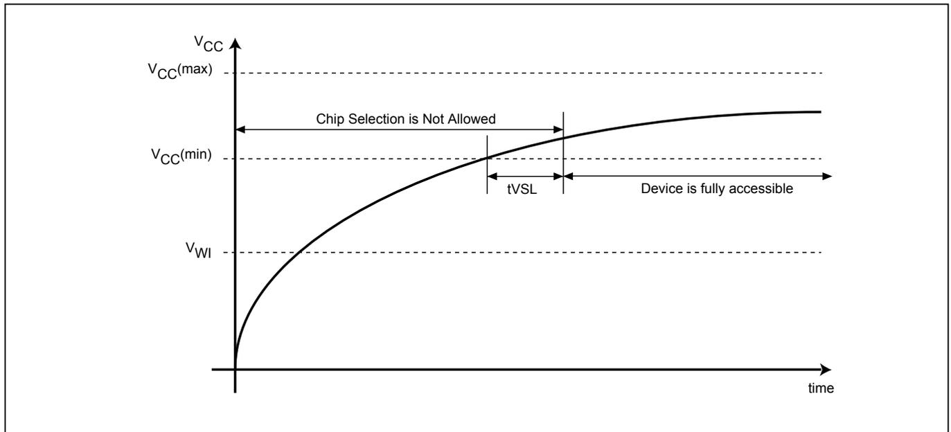
**Figure 85. Power Up/Down and Voltage Drop**
