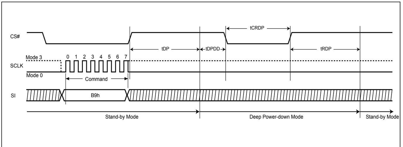
**Figure 54. Deep Power-down (DP) Sequence and Release from Deep Power-down to enter Standby Mode Sequence (QPI Mode)**
