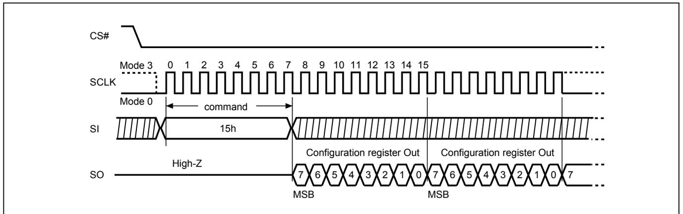
**Figure 20. Read Configuration Register (RDCR) Sequence (QPI Mode)**
