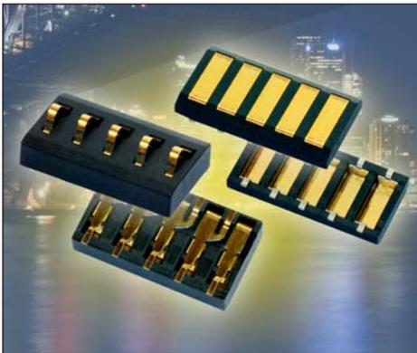
This unique battery or removable module style connector is different from most others in that it allows for the pluggable device to be swiped or connected from either direction. The spring contact offers enhanced contact deflection range over existing connectors in the market with a full 1.4mm of travel after contact engagement. This contact design allows the connector to absorb more of the plastic or housing tolerances making it more functional and reliable in real life applications.
